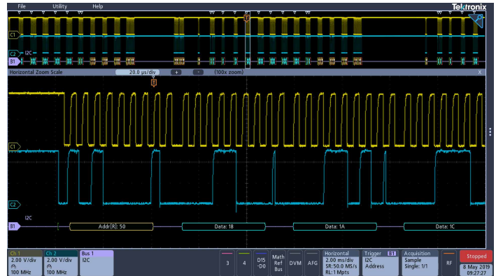
Triggering on a specific address and data packet going across an I 2 C bus. The yellow waveform is clock and the blue waveform is the data. A bus waveform provides decoded packet content including Start, Address, Read/Write, Data, and Stop.
