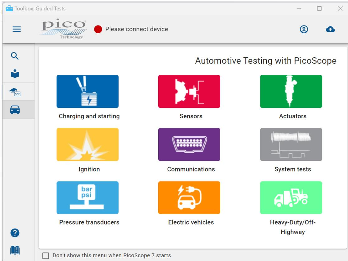
The Automotive Toolbox panel contains over 160 preset guided tests ready for you to perform on vehicles.
