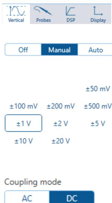
**Channel Options tabs.** Opens the **Channel Options** with options for **Vertical**, **Probes**, **DSP** and **Display**.
