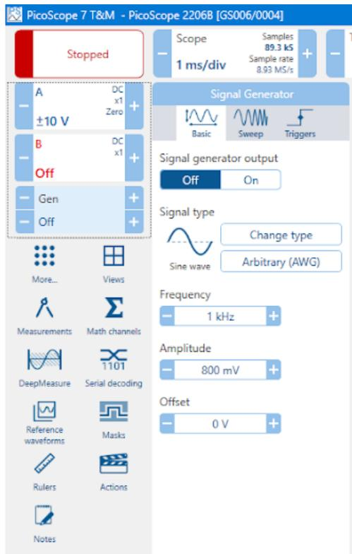
If your scope has a built-in **signal generator**, clicking the **Signal Generator** button opens the **Signal Generator options panel**
