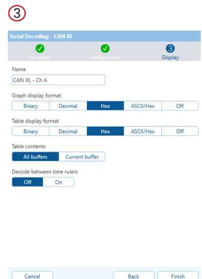
Once the data channel has been chosen and set up, configure the following options as per the CAN XL bus under test.
