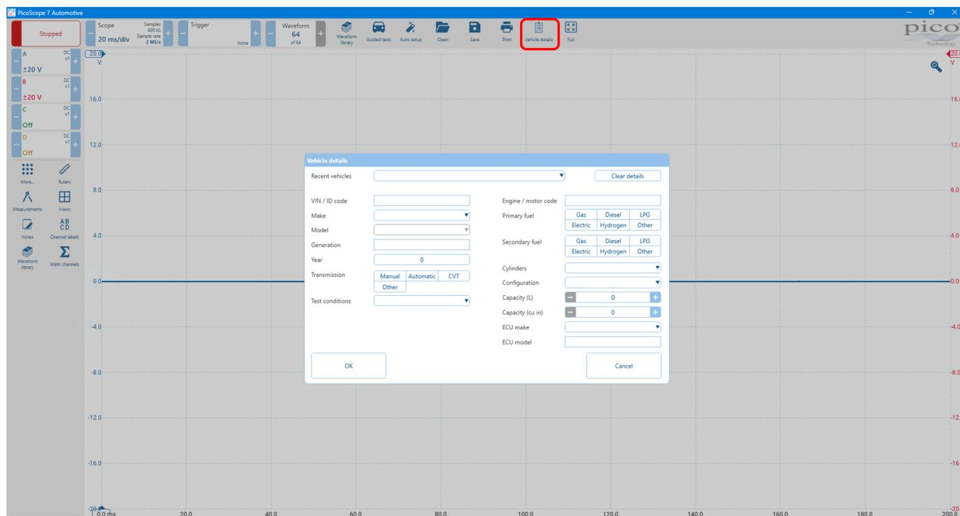
All the details you need to identify a vehicle can be entered into Vehicle details. The details can then be stored when you save your waveforms to a PicoScope data (psdata) file or upload them to the Waveform Library.
