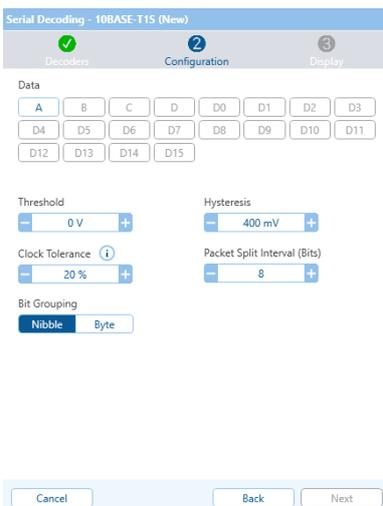
In the Configuration tab, select the corresponding PicoScope input channel for Data and provide the appropriate values for the relevant 10Base-T1S fields.
