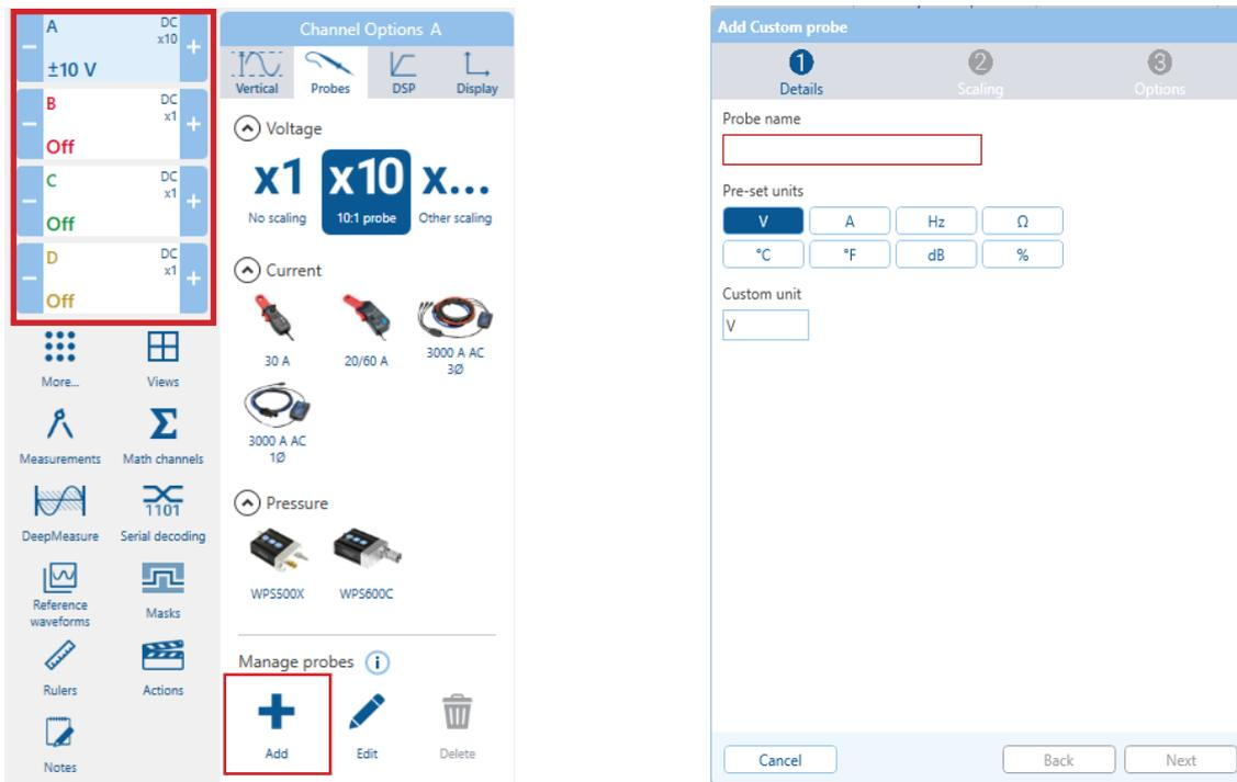
The selection of built-in probes shown may vary depending on the version of the PicoScope software that you are using. All the probes that PicoScope knows about are listed in sections according to the type of probe. The probe list is preserved between sessions, so that PicoScope will never forget your custom probes unless you delete them.
