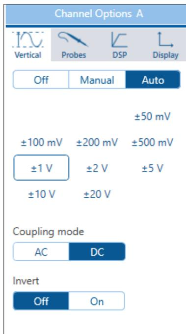
To get started, click "Auto" to turn the channel on and have PicoScope manage the input range settings according to the signal detected, or click a voltage range to manually select the input span.
