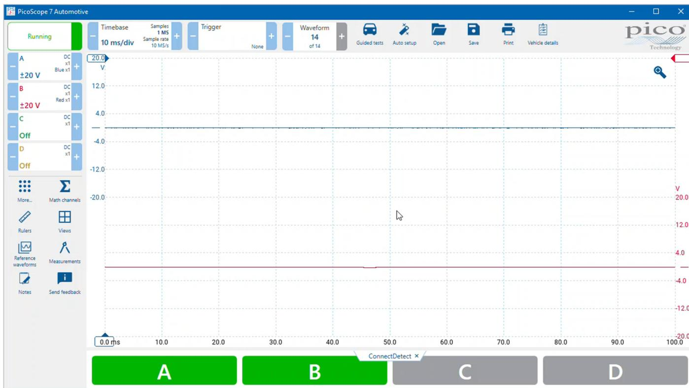
When ConnectDetect is activated, the on-screen indicator for each channel is either green, to indicate that the test probe is directly connected across a component, or red to indicate that it is not. Channels which are turned off are shown in grey, and are not tested by ConnectDetect.
