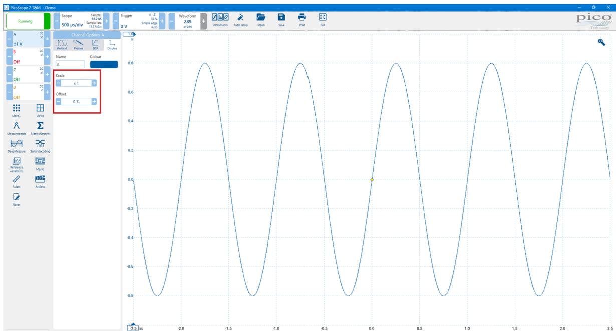
Use these tools if **Auto-arrange axes (see above)** does not give you the results you want. It allows you to position channels individually on the view (unlike the **global zooming** and **scrolling** tools, which are applied to all of the channels at the same time).
