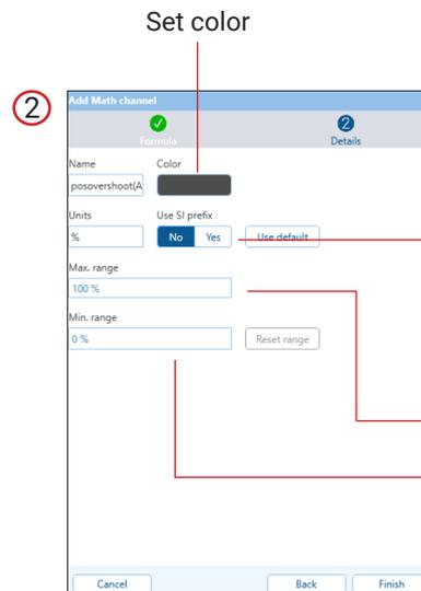
If you select Yes, then PicoScope will automatically scale your unit using the standard SI prefixes e.g. mV, V, kV. If you select "No" then PicoScope won't add a prefix
