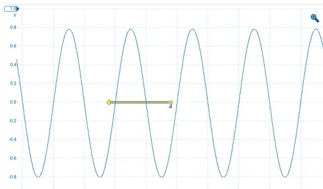
The left-hand end of the arrow indicates the trigger point, and is aligned with zero on the time axis. The right-hand end of the arrow (temporarily replacing the trigger marker) indicates the trigger reference point. You can set up a time delay using the **Trigger** controls.
