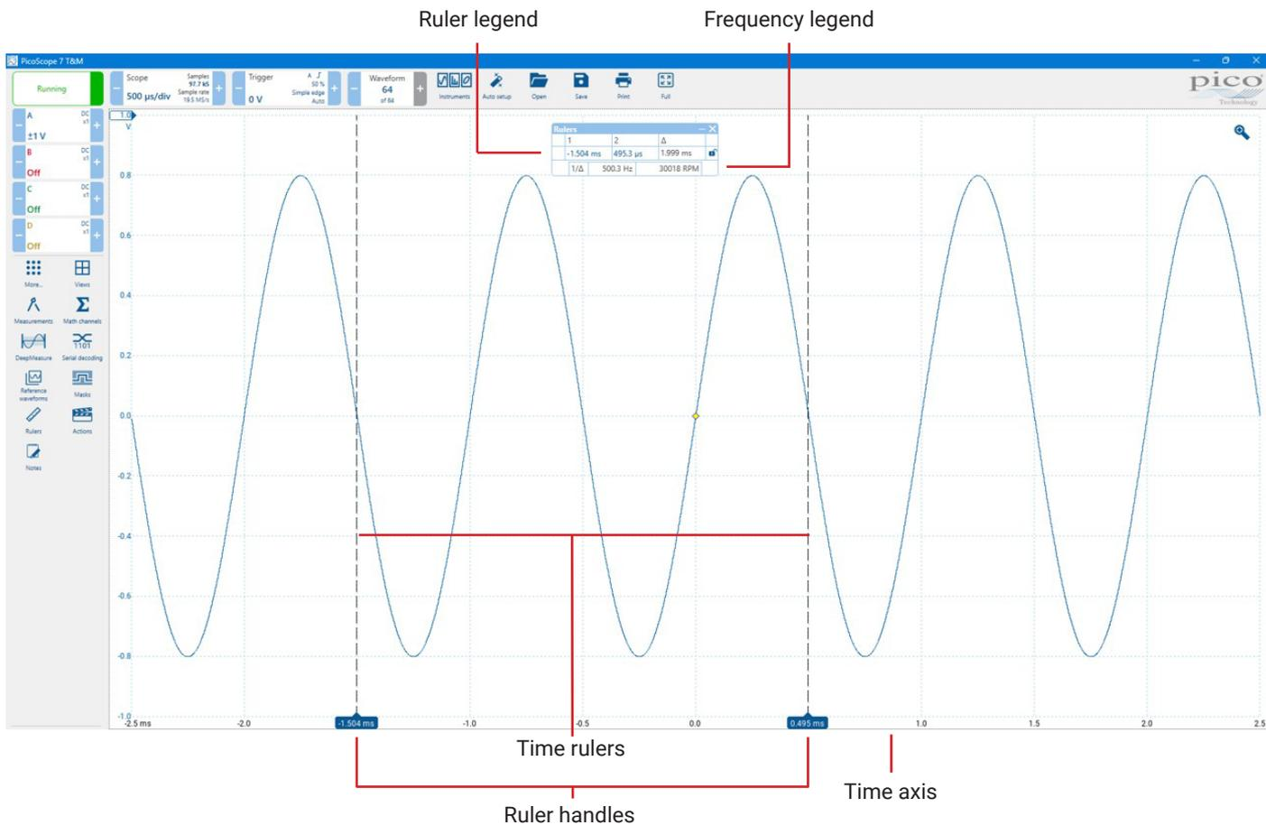
In the scope view above, the two blue rectangles on the time axis are the time ruler handles. When you drag these to the right from the bottom left corner, the time rulers appear. The rulers work in the same way on a spectrum view, but the ruler legend shows their horizontal positions in units of frequency rather than time.
