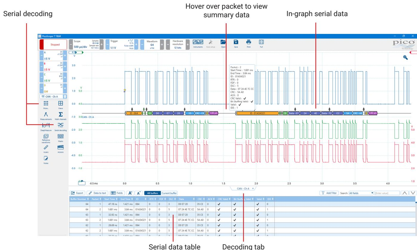
To start decoding your data, click **More... > Serial Decoding** or use the side bar. There are many different protocols available, and the data can be viewed in Graph or Table formats, or both. You can simultaneously decode multiple channels in different formats, and switch between them using the Decoding tabs.
