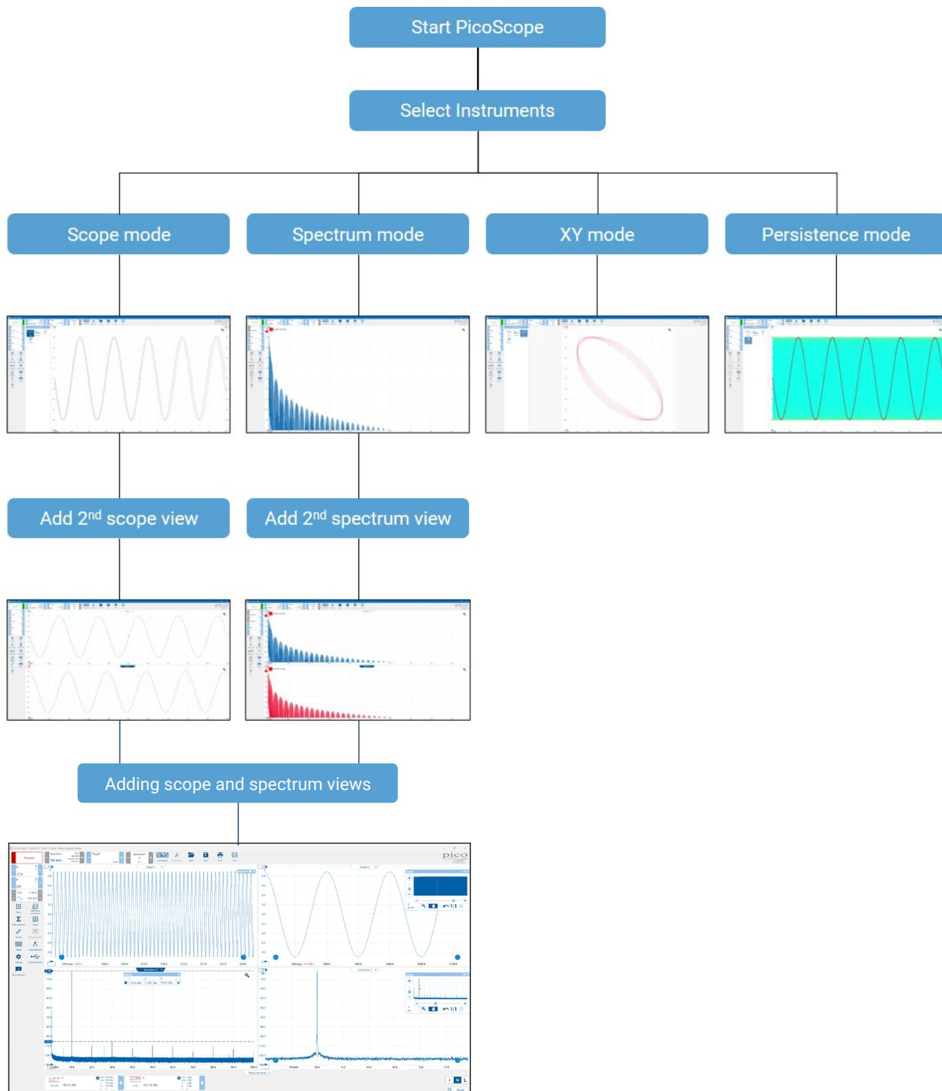
The example above is showing how you might select Instruments and open additional views in PicoScope
