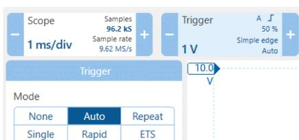
The trigger mode control tells the scope whether to wait for a trigger condition and what to do next. None, Single, Repeat and Auto modes are described in 5.3.1 Trigger Controls. Depending on the PicoScope model and timebase settings, certain PicoScope models have special modes including Rapid and ETS (Equivalent Time Sampling).
