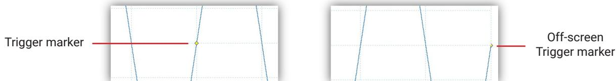
The height of the marker on the vertical axis shows the level at which the trigger is set, and its position on the time axis shows the time at which it occurs.
