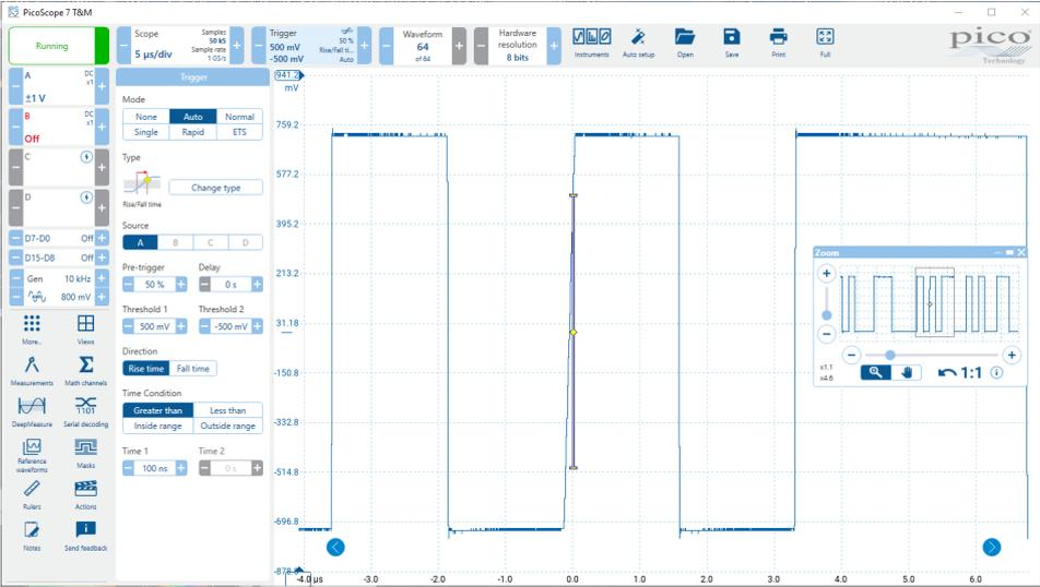
In this example above the rise time trigger was set to trigger on rising edges which transitioned from -500 mV to +500 mV in greater than 100 ns. It ignored the rising edges which were faster than 100 ns, and the falling edges regardless of their rate, and triggered only on the slower rising edge.
