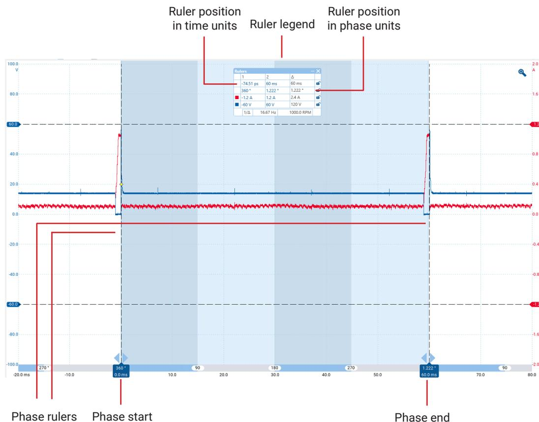
In the Scope view above, the two Phase rulers have been dragged into place to mark the start and end of a cycle.
