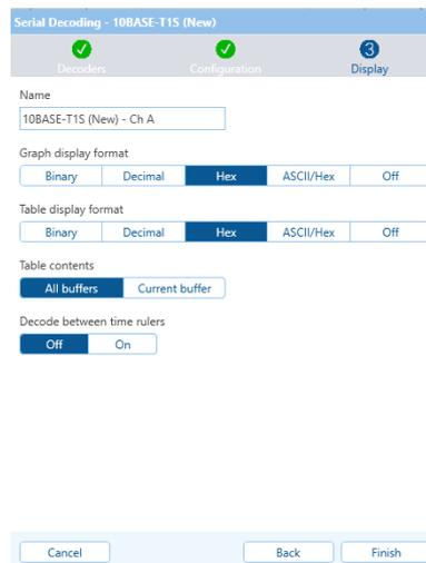
In the Display tab, select the desired Graph and Table display format options to display 10BASE-T1S packets in the appropriate locations.
