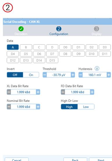
Select the corresponding PicoScope input channel for the CAN XL data signal. The data source may be the CAN XL TXD signal, CAN H, or CAN L from the differential bus.
