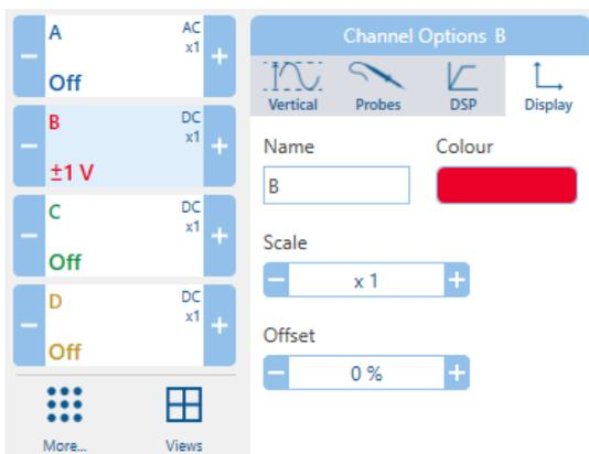
**Channels** the trace color for each scope channel can be set here.
