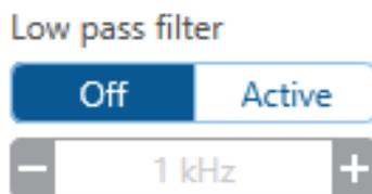
**Lowpass filtering** is useful for rejecting noise. The split screenshot below shows the effect of applying a 1 kHz lowpass filter on a noisy signal. The underlying shape of the signal is preserved but the high-frequency noise is eliminated:
