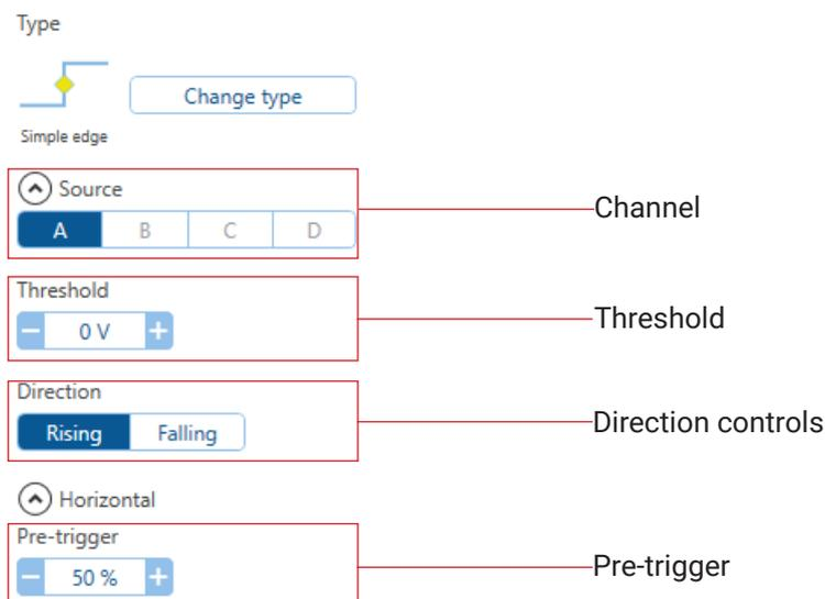
**Channel** - the input to trigger on. This can be one of the analog input channels, or a digital input pin on MSOs, or an Ext or AuxIO trigger input if available.
