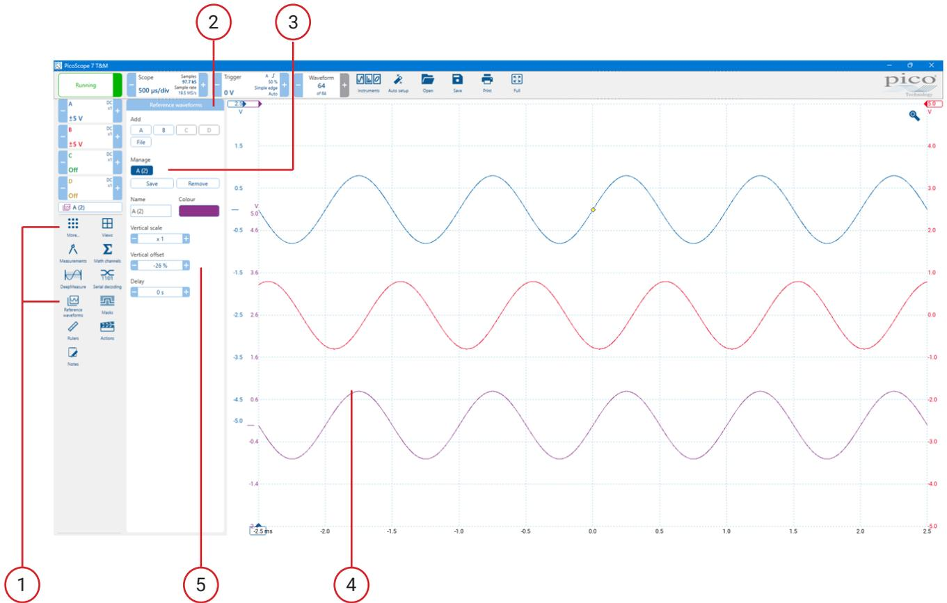
1. **More... > Reference waveforms** command or use the side bar. Click this to open the Reference Waveforms options panel, shown in the image above.
