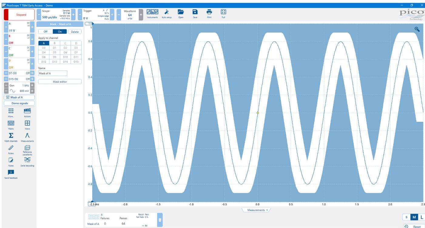
4. PicoScope stops capturing when you enter the **Mask dialog**, so click the **Stop/Running** button to restart. If any captured waveform fails to fit inside the mask, the offending parts are drawn in a contrasting color. The **Measurements** button shows the number of failures:
