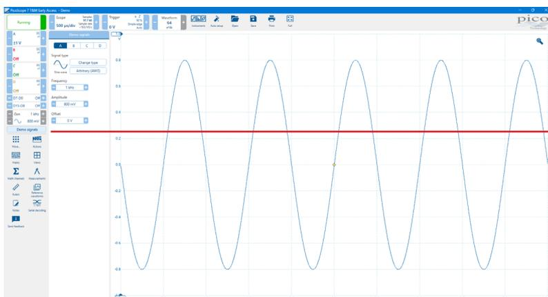
Once the demo version is running click the **Demo signals** button that appears on the left hand side. This will give you access to a range of simulated signals that are useful for evaluation of PicoScope 7 functions and for education purposes.
