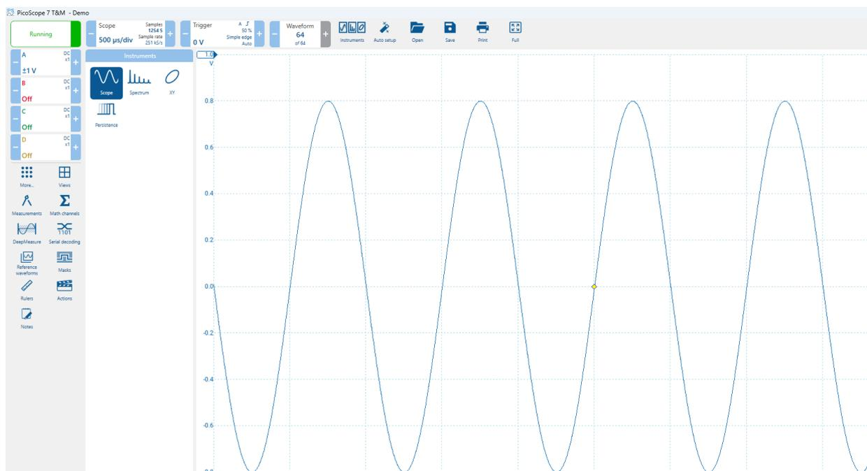
A scope view (shown above) shows the data captured from the scope as a graph of signal amplitude against time. A scope view shows you one or more waveforms with a common horizontal time axis, with signal level shown on one or more vertical axes.
