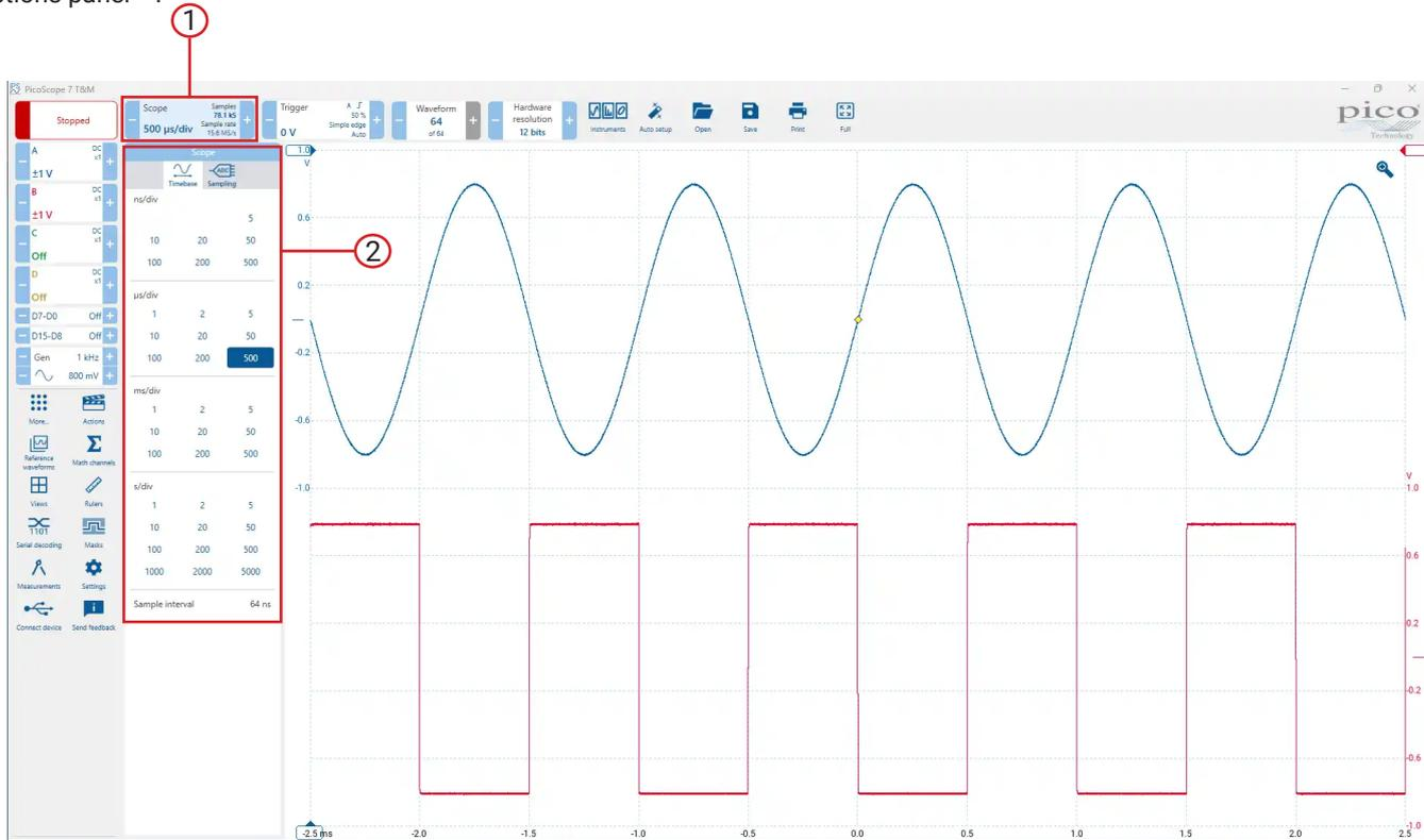
To change the Sampling settings, click Sampling <sup>(3)</sup> to adjust the Sampling mode priority, Target number of samples, Progressive mode and Previous progressive waveform from the Sampling options panel.
