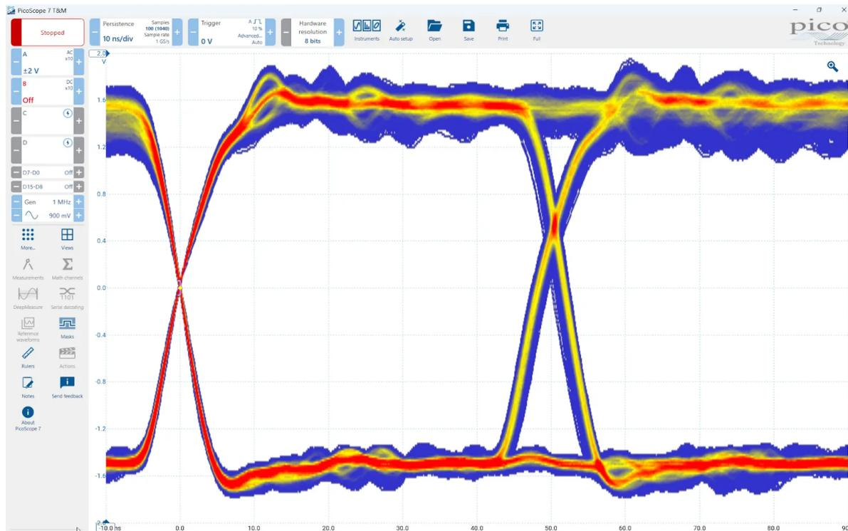
The colors indicate how frequently each point in the waveform occurs. Red is used for the most frequently occurring parts of the signal, with yellow for intermediate and blue for the least frequently occurring. In the example above, the waveform spends most of its time in the red region, but noise causes it to wander occasionally into the blue and yellow regions.
