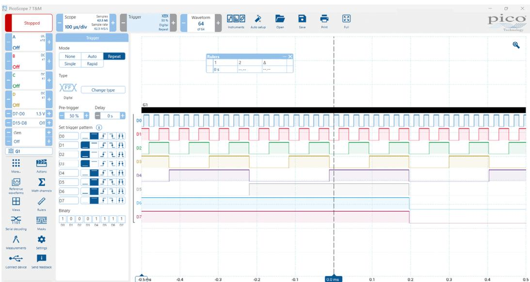
The Digital trigger can be fed into the Logic trigger, described in section **Logic trigger**, to allow you to look for composite conditions of the analog and digital inputs.
