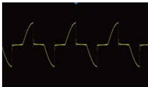
TrailingEdge phase dimming
