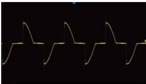
LeadingEdge phase dimming
