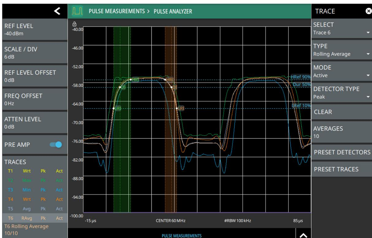
1. Clear/Write and Peak Detection: This is the default trace setting. The trace is cleared during each sweep and the largest measurement point is used for each display point.
