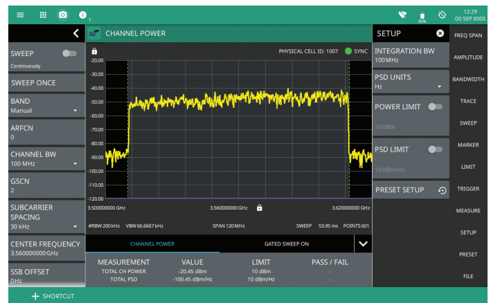
5G Channel Power Results in 5G Mode
