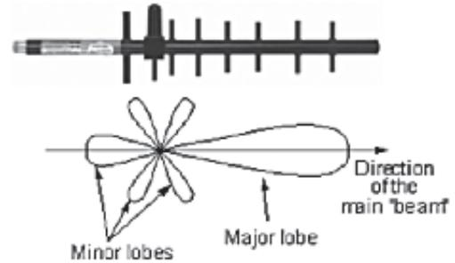
Figure 2. A Yagi antenna and its pattern
