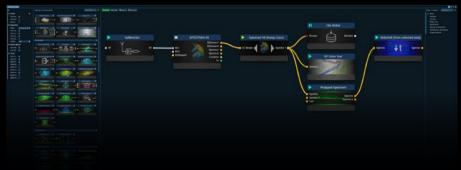
Modify, arrange and connect blocks to analyze data using drag & drop. Blocks have connectors with colors and labels representing supported data types.
