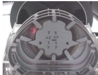
Figure 2-7. Macrobend detected with VFL
