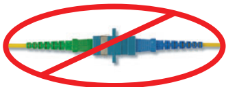
Figure 2-3. UPC connector connected with APC connector
