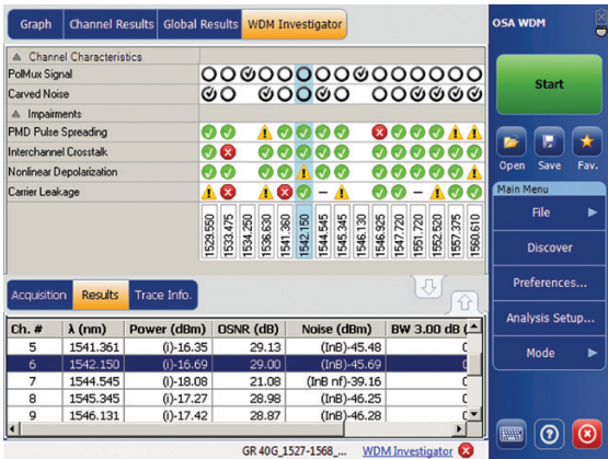
Figure 111. WDM Investigator reading showing a non-linear depolarization contributing to extended noise (OSNRe).
