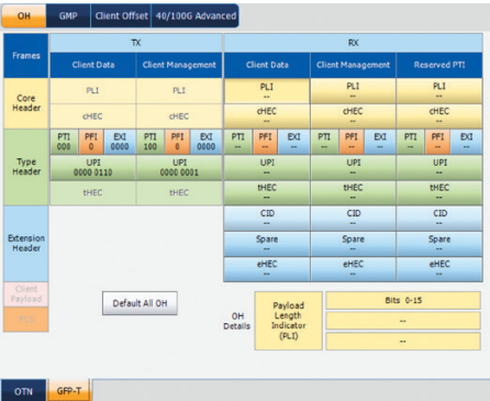
Figure 50. GFP-T overhead-byte analysis interface on EXFO's FTBx-88200NGE OTN analyzer.
