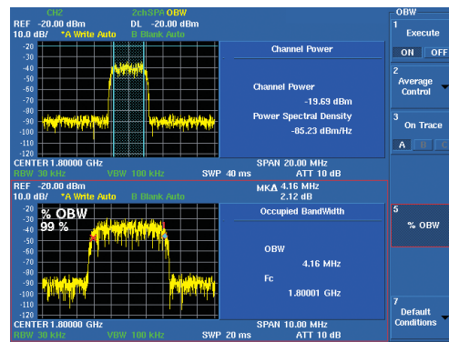
Simultaneous measurement of POWER and OBW
