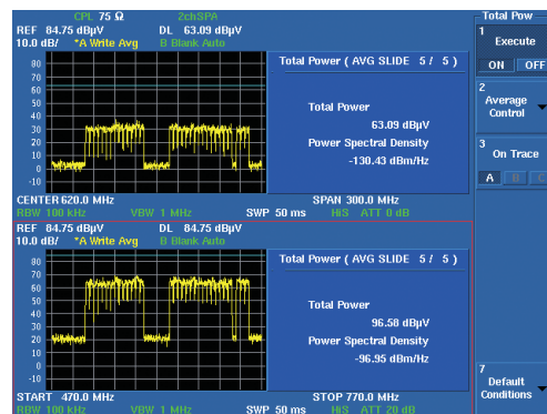
Simultaneous measurement of input/output for feed-forward amp
