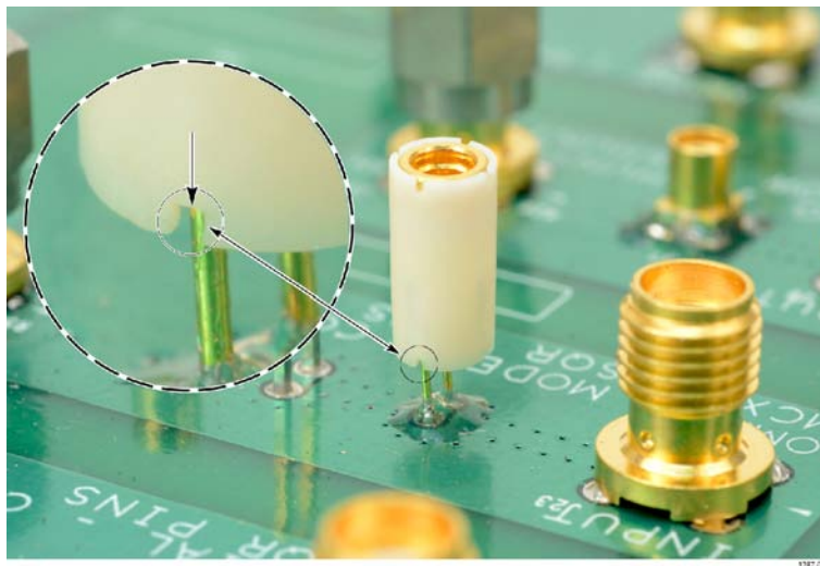
Figure 30: Lining up the MMCX-to-0.062-inch (1.57 mm) adapter on the circuit board
