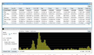
Cumulative statistics provides timestamps for Min, Max values as well as Peak to Peak, Average and Standard deviation over multiple acquisitions, further extending the analysis. Histogram shows you outliers on the right and left
