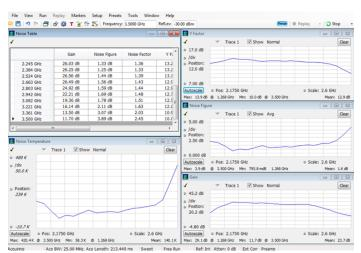
Noise Figure and Gain measurements (Option 14) help you to quickly and easily measure your device using the RTSA and a noise source. This image shows the measurement summary table with graphs of noise temperature, gain, noise figure and Y-
