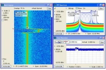
Trigger and Capture: The DPX Density<sup>™</sup> Trigger monitors for changes in the frequency domain, and captures any violations into memory. The spectrogram display (left panel) shows frequency and amplitude changing over time. By selecting the point in time in the spectrogram where the spectrum violation triggered the DPX Density™ Trigger, the frequency domain view (right panel) automatically updates to show the detailed spectrum view at that precise moment in time.
