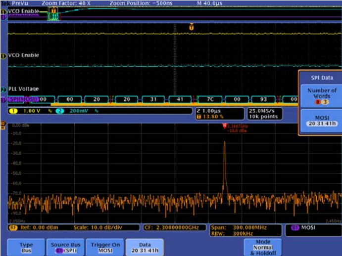
Capture – Triggering on a specific transmit data packet going across a SPI bus. A complete set of triggers, including triggers for specific serial packet content, ensures you quickly capture your event of interest.
