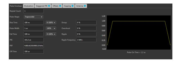
**NOTE.** The available Pulse Envelope parameters depend on the selected pulse shape. Not all parameters are available for all pulse shapes.
