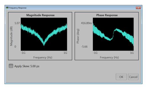
When applying an I/Q correction file you can choose either a single IQ correction file or correction files for I and Q. The Frequency Response screen shows plot information and provides Advanced Options to apply a Gaussian filter or remove Sin(x)/x distortions. When selecting I and Q correction files, separate files for I and Q are shown in the Frequency Response window.
