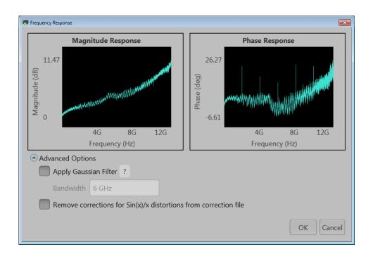
If applying an I/Q correction file (to a pair of I and Q waveforms), the Frequency Response screen shows plot information and provides Advanced options to apply a skew.
