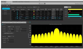
The Tektronix Environment signals plug-in is a simple and flexible tool to create real world scenarios for commercial, electronic warfare, and simulations for monitoring and receiver testing. The plug-in integrates into the SourceXpress waveform creation platform, and the AWG70000 series and AWG5200 series arbitrary waveform generators.
