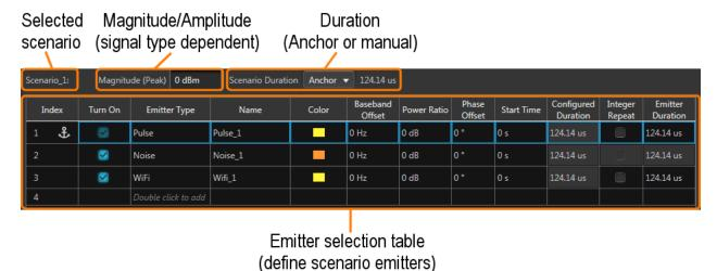
Once an emitter is added to the Scenario definition area, selecting the emitter displays its Advanced settings in tabs at the bottom of the screen.
