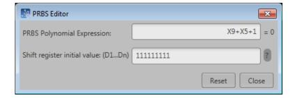
PRBS sequences are generated by a feedback shift register. The number (#) following PRBS indicates the length of the generating shift register. For instance, a shift register with 16 memory cells is required to generate a PRBS 16 sequence. The pseudo-random sequence of a PRBS generator is determined by the number of registers and the feedback.
