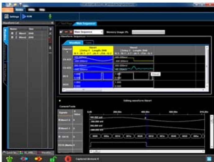
In the Multi-sequence mode, two sequences can be defined to control Channel 1 and Channel 2 (and the corresponding digital channels) separately as two units of generator.
