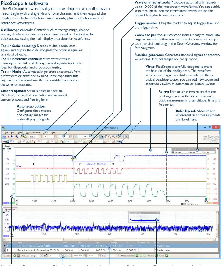
Movable axes: The vertical axes can be dragged up and down. This feature is particularly useful when one waveform is obscuring another. There's also an Auto Arrange Axes command.
