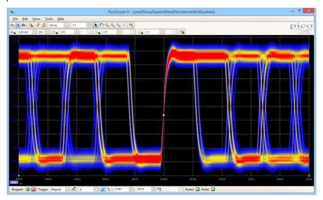
Color Persistence mode allows you to see old and new data superimposed, with new or more frequent data in a brighter color or shade. This makes it easy to see glitches and dropouts and to estimate their relative frequency. Simply click the persistence button between analog intensity, digital color, and fast display modes, or create your own custom rules.
