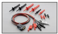
Model 3706-TLK Test Lead Kit: Includes 3706-BAN banana test leads/adapter cable and plugin test lead accessories. Test lead accessories include: 4 spring hook probes, 2 needle test probes, 4 safety plug adapters, and carrying case.
