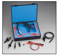
Model 2187-4 Low Thermal Test Lead Kit: Includes an input cable with banana terminations, banana extensions, sprung-hook clips, alligator clips, needle probes, and spade lugs to connect the Model 2182A to virtually any DUT. The kit is also used to connect the Model 2182A directly to the Model 622X guard to improve response time for pulsed measurements or to reduce errors when measuring high impedance devices.
