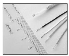
**Model 8681 Low Cost RTD:** This inexpensive RTD has small size  $(0.09 \text{ in} \times 0.09 \text{ in})$  and fast thermal response time.  $100\Omega$ ,  $0.385\%^{\circ}\text{C}$  element. Meets or exceeds DIN 43760-1980-A, IEC 751:1983-A, BS1904: 1984-A, and JIS C1604-1981-0.2. Can be used with Model 8680 RTD Input Probe Adapter. Measures from  $-200^{\circ}$  to  $+600^{\circ}\text{C}$ .
