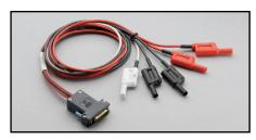
Model 3706-BAN: 1.4m (4.6 ft) banana test leads/adapter cable for Model 3706A mainframe with high performance multimeter option. Provides direct connection to high performance multimeter utilizing rear panel backplane connector. Safety banana connections to HI, LO, Sense HI, Sense LO, and AMP.
