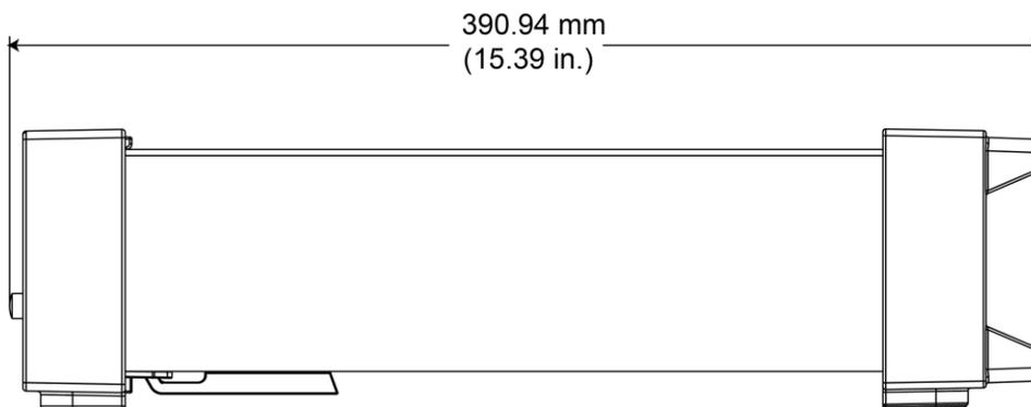
The following figures show the dimensions when the handle and bumpers have been removed.
