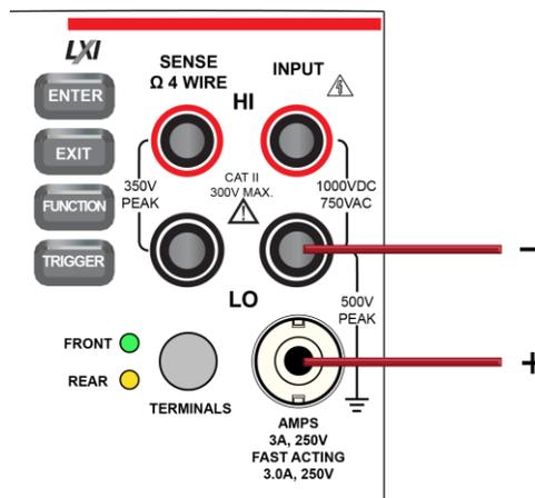
**Figure 98: Rear panel connections: Digitize current measurement (current below 3 A)**
