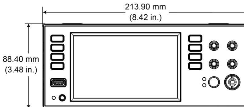
**Figure 5: DMM6500 side dimensions with bumpers removed**
