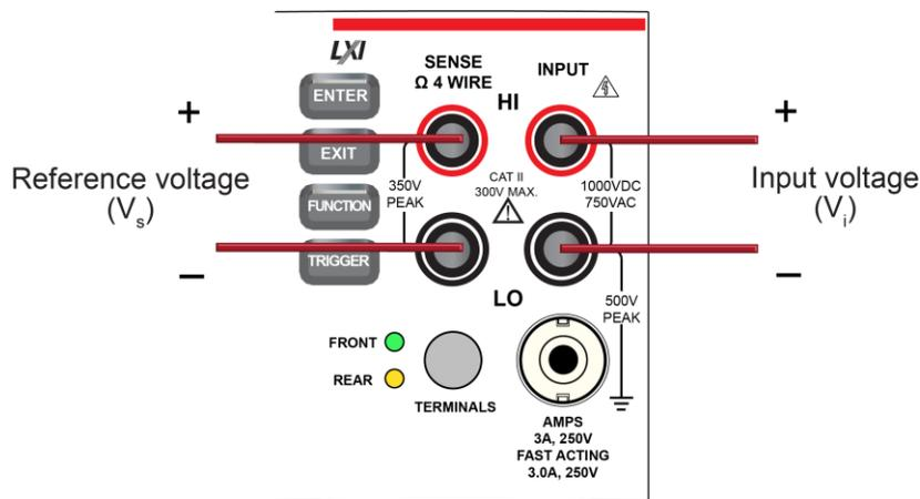
Figure 94: Rear panel connections: DC voltage ratio measurement
