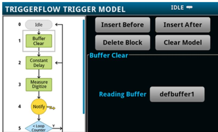
To see the parameters that you can change from the front panel, select a block in the trigger model diagram. The available options change depending on the type of block you select.
