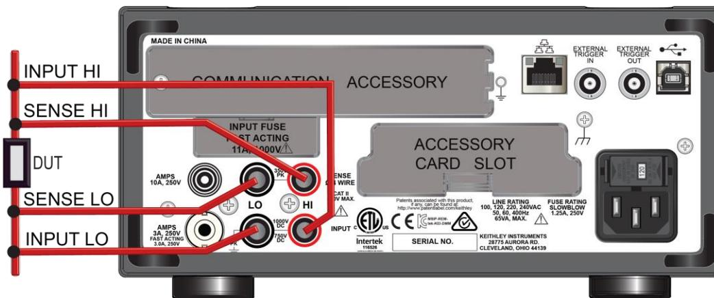
**Figure 74: DMM6500 front-panel 4-wire remote sense connections**
