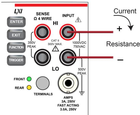
Figure 76: Rear panel connections: 2-wire resistance measurement
