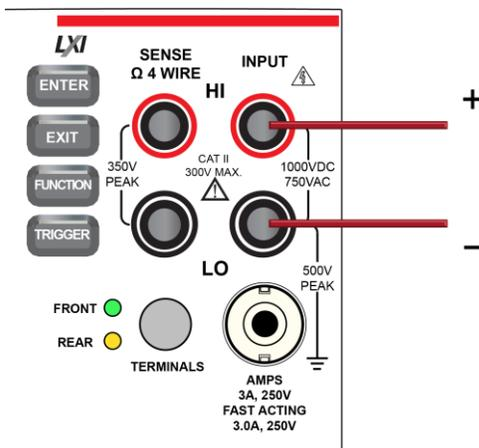
Figure 90: Rear panel connections: Capacitor measurement
