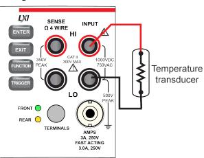
Figure 76: 4-wire RTD measurement
