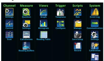
Figure 50: DAQ6510 main menu - front terminals selected
