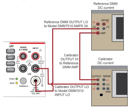
Figure 176: DC current verification 10 µA to 100 mA range
