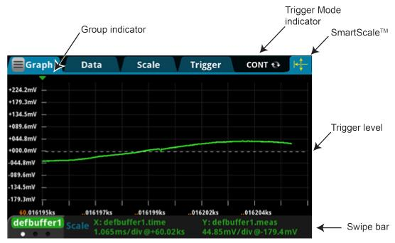
Figure 52: DAQ6510 graph tab
