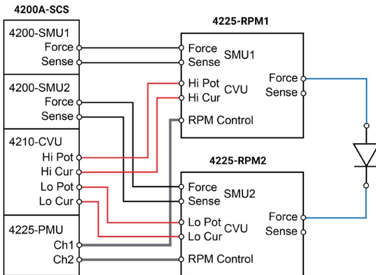
Both the red cables (supplied with the CVU) and the blue cables (supplied with the optional 4210-MMPC cable kits) are 100 Ω. You can do [remote sensing](#) (on page 5-25) using the optional 4210-MMPC cable kits with the RPMs.
