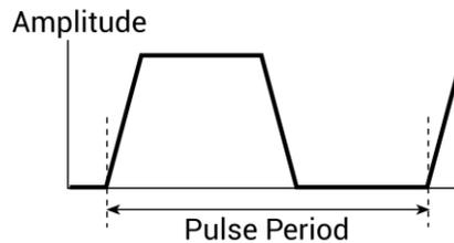
The pulse period setting takes effect immediately during continuous pulse output. Otherwise, the period setting takes effect when the next trigger is initiated. The `pulse_trig` command is used to trigger continuous or burst output.
