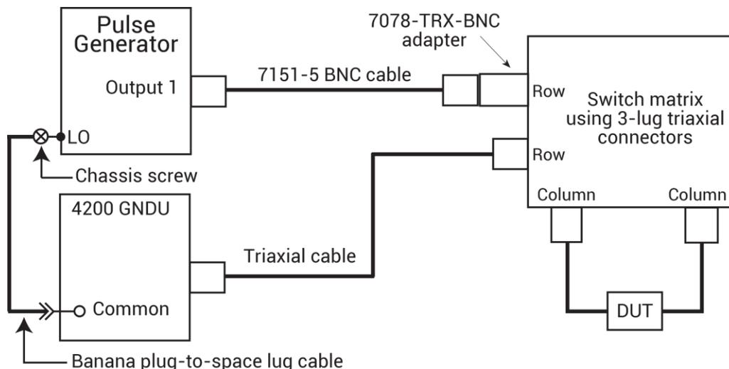
The following figure shows the actual pulse output signal path through the switch matrix to the device under test (DUT), and back to the pulse generator. A more detailed look at signal paths is provided in [Using Switch Matrices](#) (on page A-1).
