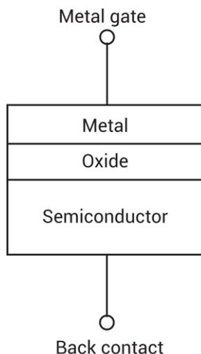
The most important property of the MOS capacitor is that its capacitance changes with changes to applied voltage. As a result, the modes of operation of the MOS capacitor change as a function of the applied voltage. As a DC sweep voltage is applied to the gate, it causes the device to pass through accumulation, depletion, and inversion.
