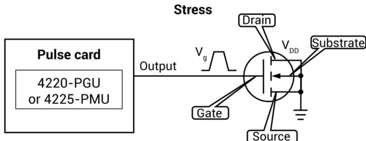
Figure 322: AC Pulse stress-measure — hardware setup block diagram for measure
