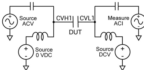
The following settings source AC drive voltage and DC bias voltage to the CVL1 terminal. AC current is measured at CVH1.
