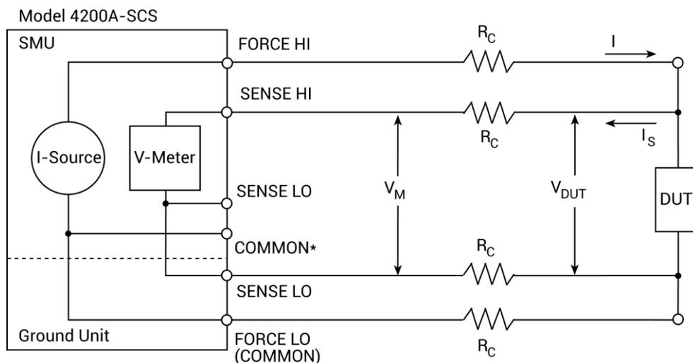
\* Common terminal on the SMU is the outside shield of the triaxial connector.
