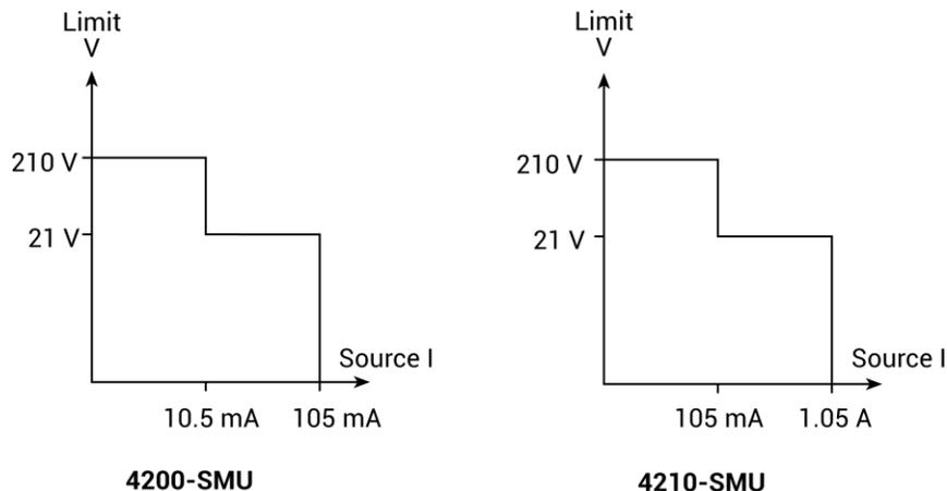
The next figure shows the limit lines for the I-source. The current source limit line represents the maximum source value possible for the selected current source range. For example, the current source limit line is at 105 mA on the 100 mA current source range. The voltage compliance limit line represents the actual compliance that is in effect.
