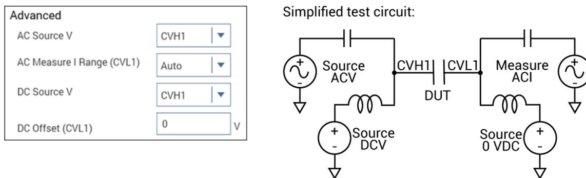
You can change the configuration to source AC voltage to CVL1 and DC source voltage to CVH1 while measuring AC current at CVH1, as shown in the following figure.
