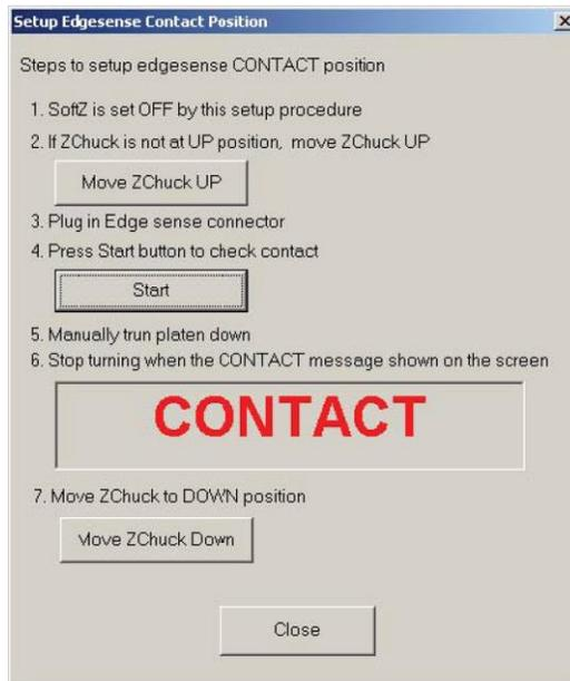
3. Move the Z Chuck up to confirm contact condition using the **Contact** icon on the toolbar.
