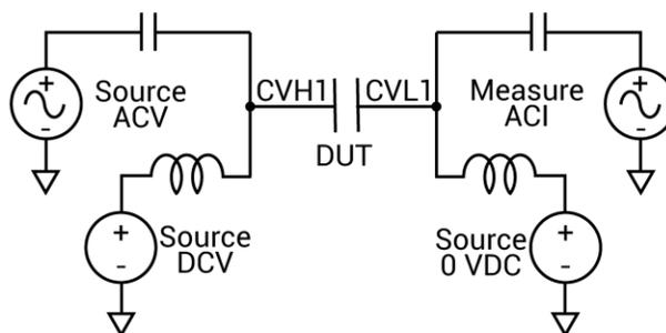
You can change the configuration to source AC voltage to CVL1 and DC source voltage to CVH1 while measuring AC current at CVH1, as shown in the following figure.
