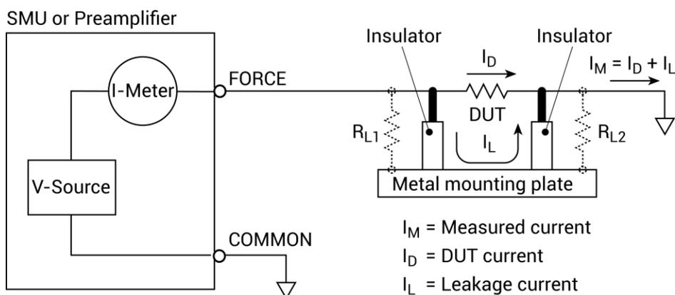
In the following figure, the driven GUARD is connected to the metal guard plate for the insulators. Since the voltage on either end of  $R_{L1}$  is the same (0 V drop), no current can flow through the leakage resistance path. As a result, the SMU or preamplifier measures only the current through the DUT.
