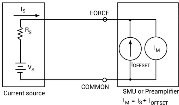
Offset currents can also be generated externally from such sources as [triboelectric](#) (on page 13-16) and [piezoelectric effects](#) (on page 13-17). As shown in the next figure, the external offset current also adds to the source current, and the SMU again measures the sum of the two. These external offset currents can be suppressed manually by subtracting them using the Formulator. For more information, refer to [The Formulator](#) (on page 6-290) and Analyze data using the Run tab.
