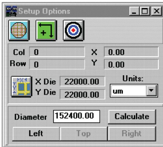
6. Click Set X, Y die size button in the Setup Options window. The Set X, Y Die size dialog box opens.
