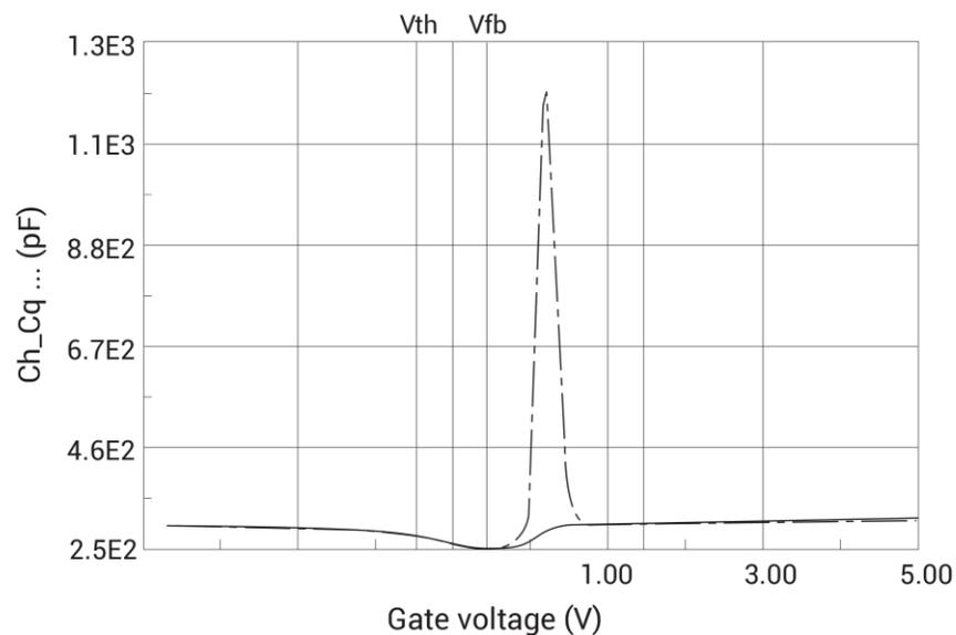
Calculation of the mobile charge concentration could come from the measured  $V_{GS}$ ,  $C_q$ , and  $C_h$  data. Alternatively, one can calculate the concentration graphically from the displayed simultaneous C-V curves.
