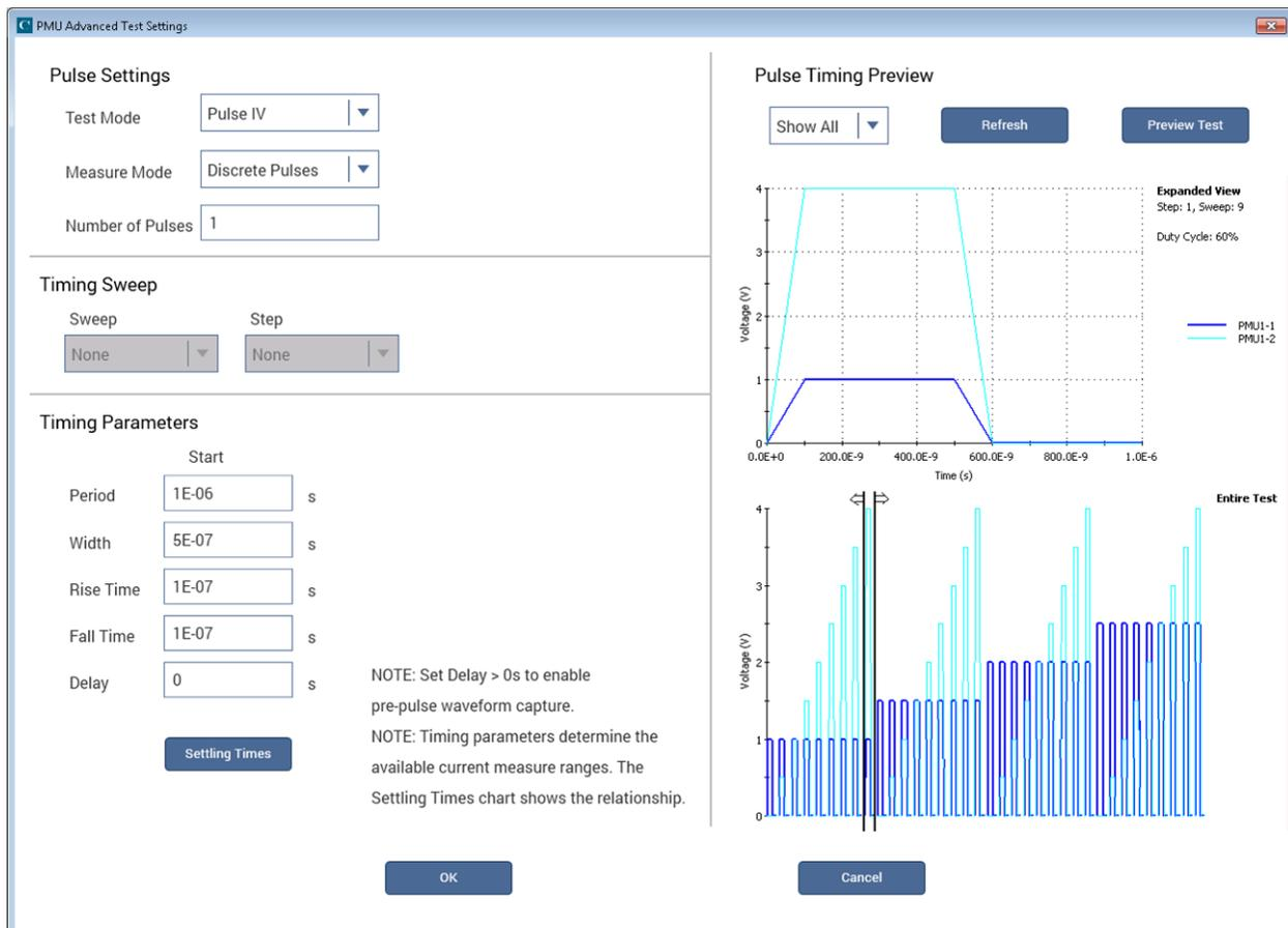
Changing the number of pulses to three (instead of one) and only displaying one channel (PMU1-1, instead of Show All), changes the preview of the waveform (see next figure). Each point in the step now uses three periods, so there are three pulses shown in the Expanded View. In the Expanded View, the x-axis shows the time in seconds. This is three times longer than the Expanded View graph when number of pulses is set to one (see previous figure).
