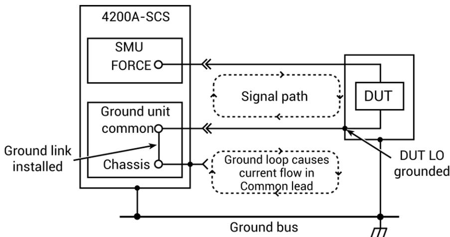
Figure 598: Eliminating ground loops
