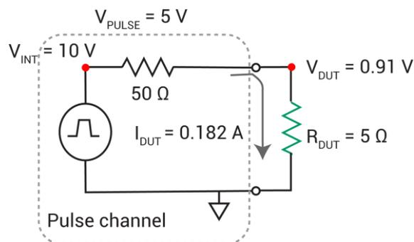
This figure shows a 5 V pulse into a 5 Ω DUT load.
