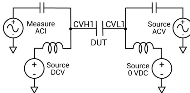
Another configuration sources AC drive voltage to the CVH1 terminal and sources DC bias voltage to the CVL1 terminal. AC current is measured at CVL1.
