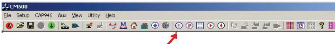
5. Click the **To First Site** button to move the prober to the first programmed site for testing. Make sure the Subsite (template) is disabled here.
