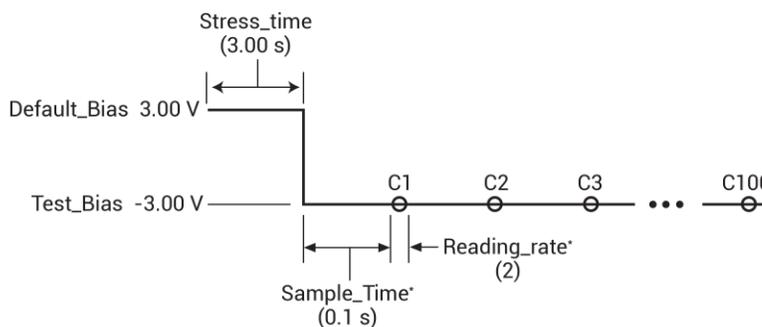
\* The time interval between reading samples is the sum of the set Sample Time and the Reading Rate time. The Reading Rate time for Reading\_rate2 is 1/18 s (0.0555 s). Therefore:
