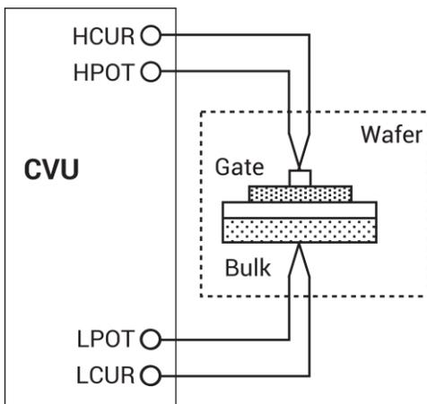
[4210-CVU connections](#) (on page 4-7) provides details on connections to a semiconductor wafer. Use only the supplied (red) 100  $\Omega$  SMA cables for connections to the 4210-CVU. Be sure that all SMA cables are the same length.
