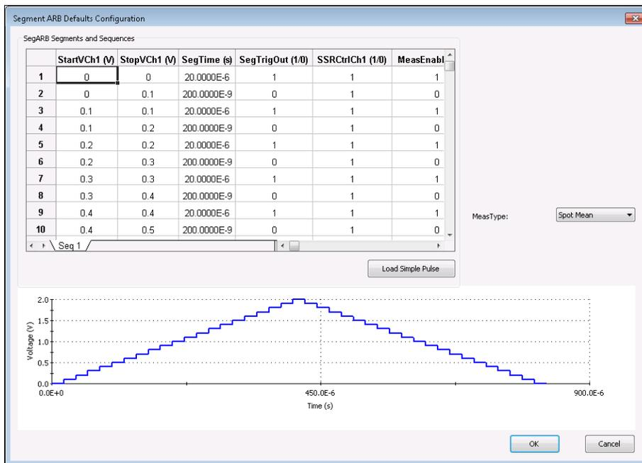
Figure 301: Two-sequence Segment Arb waveform
