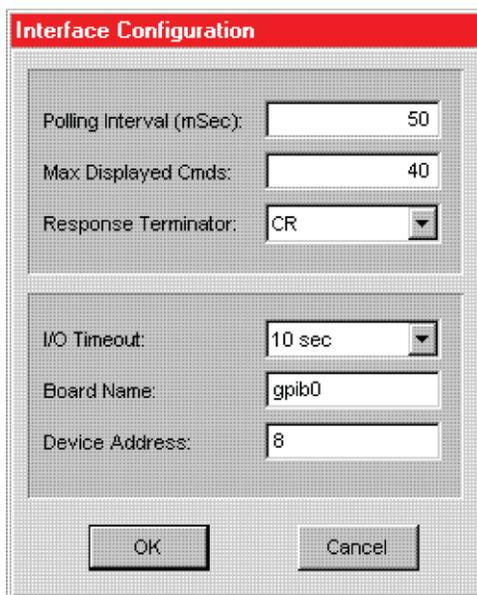
10. GPIB only: Ensure that the GPIB address matches the address in the configuration file.
