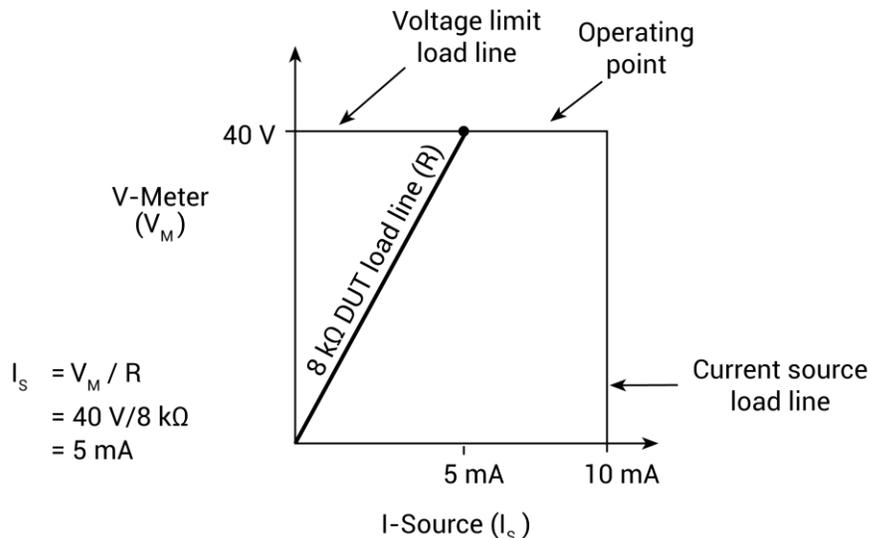
Notice that as resistance increases, the slope of the DUT load line increases. As resistance approaches infinity (open output), the SMU will source virtually 0 mA at 40 V. However, as resistance decreases, the slope of the DUT load line decreases. At zero resistance (shorted output), the SMU will source 10 mA at virtually 0 V.
