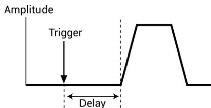
The maximum pulse delay that can be set depends on the presently set period for the pulse. For example, if the period is set for 500 ns, the maximum pulse delay that can be set is 490 ns (500 ns – 10 ns = 490 ns).
