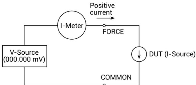
NOTE: Positive current flowing out of FORCE results in positive (+) measurements.
