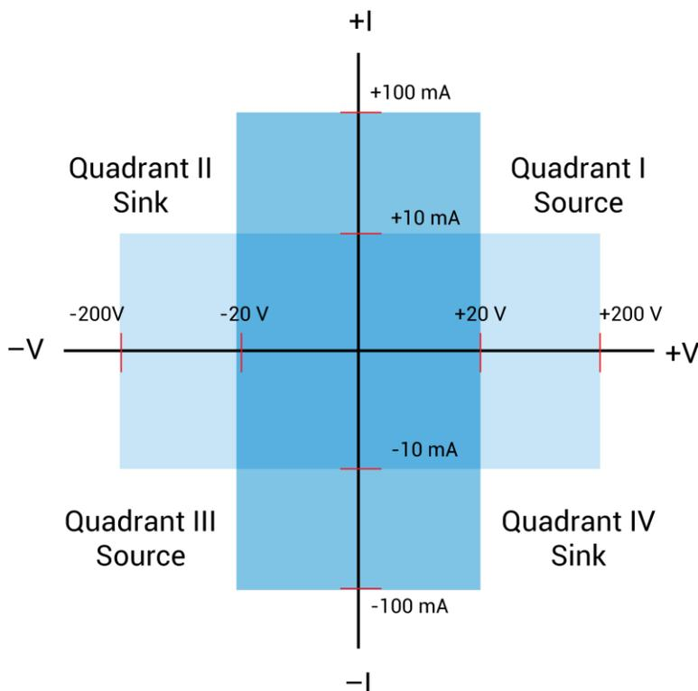
**421x-SMU with 4200-PA:** In the next figure, the 1 A, 20 V and 100 mA, 200 V magnitudes are nominal values. The actual maximum output magnitudes of the 421x-SMU and 4200-PA are 1.05 A, 21 V and 105 mA, 210 V. Note that the boundaries are not drawn to scale.
