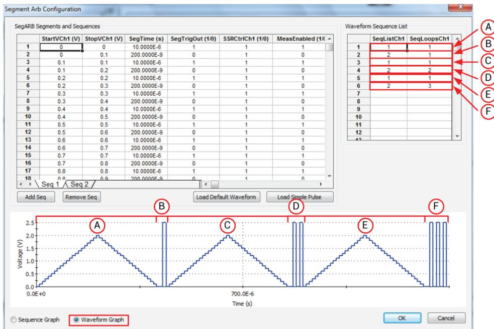
The graph of the measurement of a two-sequence Segment Arb with looping, from UTM pmu-segarb-complete in the pmu-dut-examples project, is shown in the following figure.
