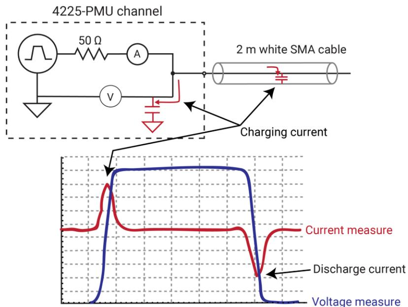
The setup used to generate these waveforms is shown in the previous figure, and also shows the capacitance and the charging effect (red arrows) seen during pulse transitions. This setup shows a single channel of a PMU, with the supplied 2 m (6.5 ft) white SMA cable connected to the channel output. Note that the other end of the SMA cable is open (no connection).
