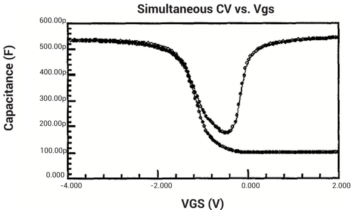
The upper flat, or accumulation region of the high frequency C-V curve defines the oxide capacitance, COX. Since most analysis relies on the ratio C/COX, it is important that you choose a start or stop voltage (depending on the sweep direction) to bias the device into strong accumulation at the start or the end of the sweep.
