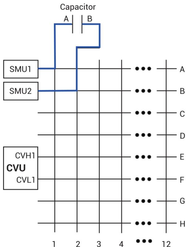
The switching matrix then connects the 4210-CVU to the capacitor, as shown in the following figure, and C-V measurements are made.
