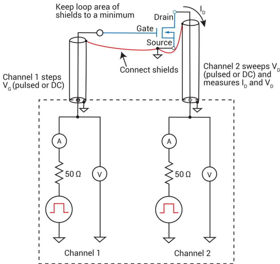
If ultra-fast I-V sourcing and measuring is required at each device terminal, then a second PMU is required for the source terminal. Up to four PMUs (eight channels) can be installed in one 4200A-SCS mainframe.
