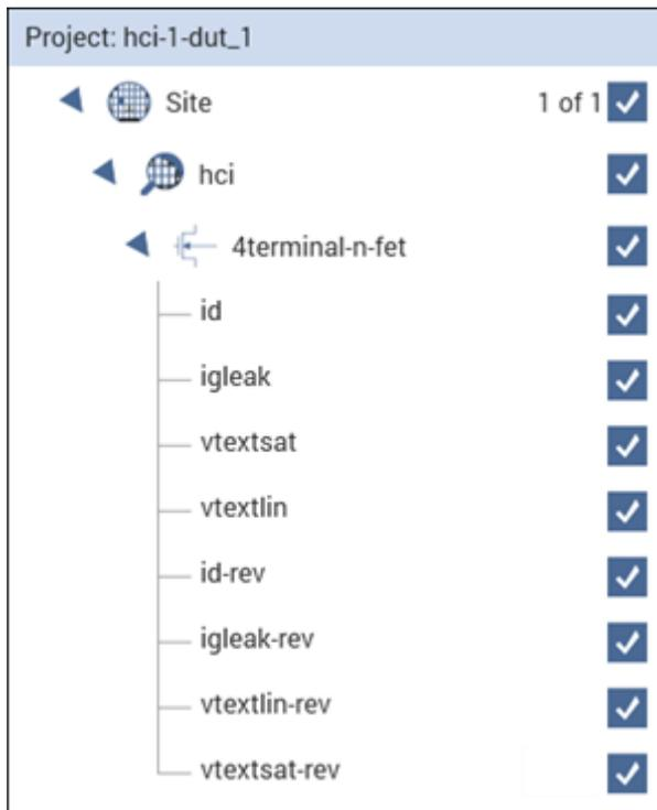
For the `hci-1-dut` project, the `hci` subsite is set up for subsite cycling using voltage stressing on the single n-channel MOSFET device (`4terminal-n-fet`). After the first pre-stress cycle to perform characterization tests, subsequent cycles voltage stress the device for a specified time before repeating the tests.
