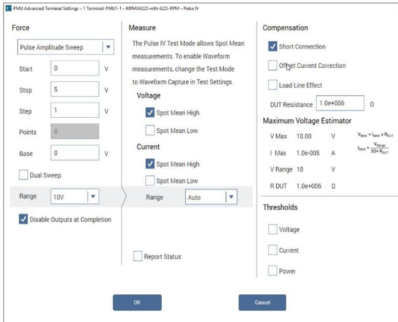
The next figure illustrates the configuration of a six-step pulse amplitude sweep. In this sweep, the PMU Advanced Settings dialog box (see previous figure) defines the test parameters.
