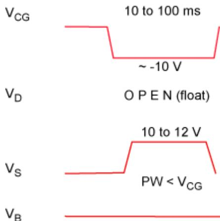
**Figure 413: Program + Erase pulse waveforms for a floating gate DUT, with separate pulse waveforms for the DUT gate, drain, source, and bulk**
