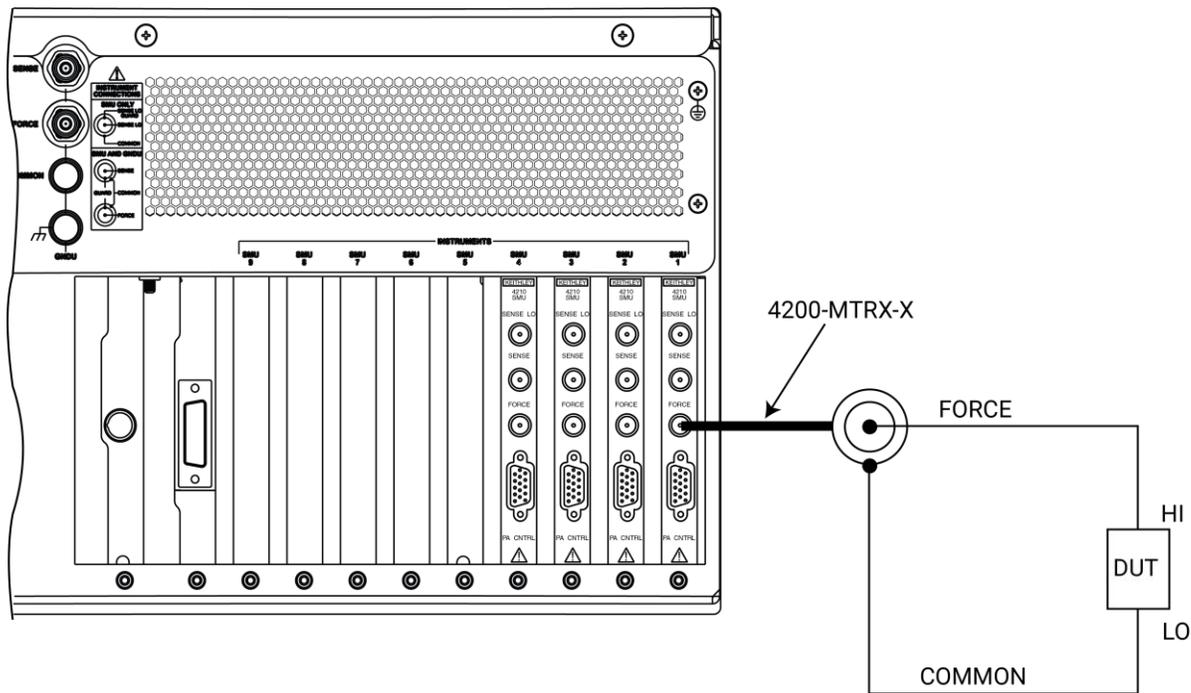
Figure 7: SMU local sense connections - equivalent circuit
