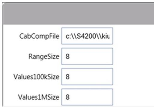
To prevent unpredictable results, the array size values for the `RangeSize`, `Values100kSize`, and `Values1MSize` arrays must be set to 8.
