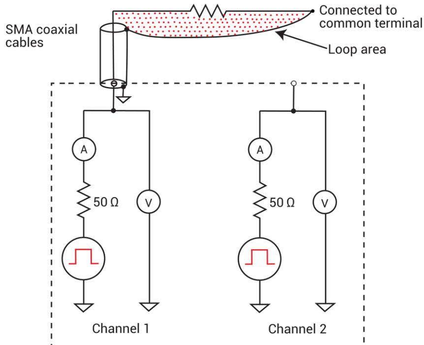
You can also connect a two-terminal device to the two channels of a PMU, as shown in the next figure. In this case, channel 1 will source/pulse voltage, and channel 2 will measure the resulting current. Make sure you connect the shields of the SMA cables close to the device under test. This method avoids problems of capacitive charging (see [PMU capacitive charging/discharging effects](#) (on page 5-53)).
