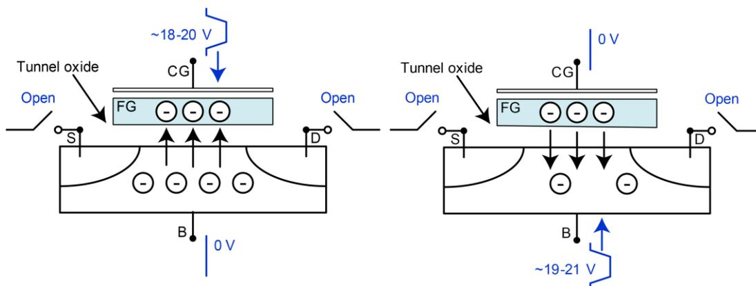
The following figure shows examples of moving charge using HCI. These conditions are examples with approximate voltage values. The pulse width and pulse height will vary depending on device structure and process details.
