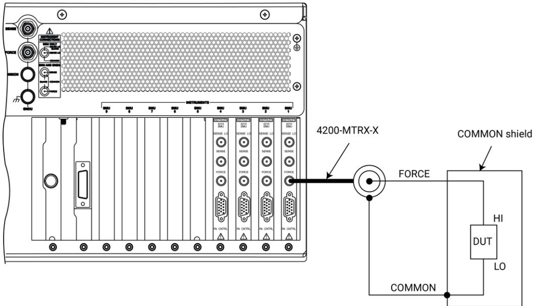
Figure 3: Device shielding basic circuit
