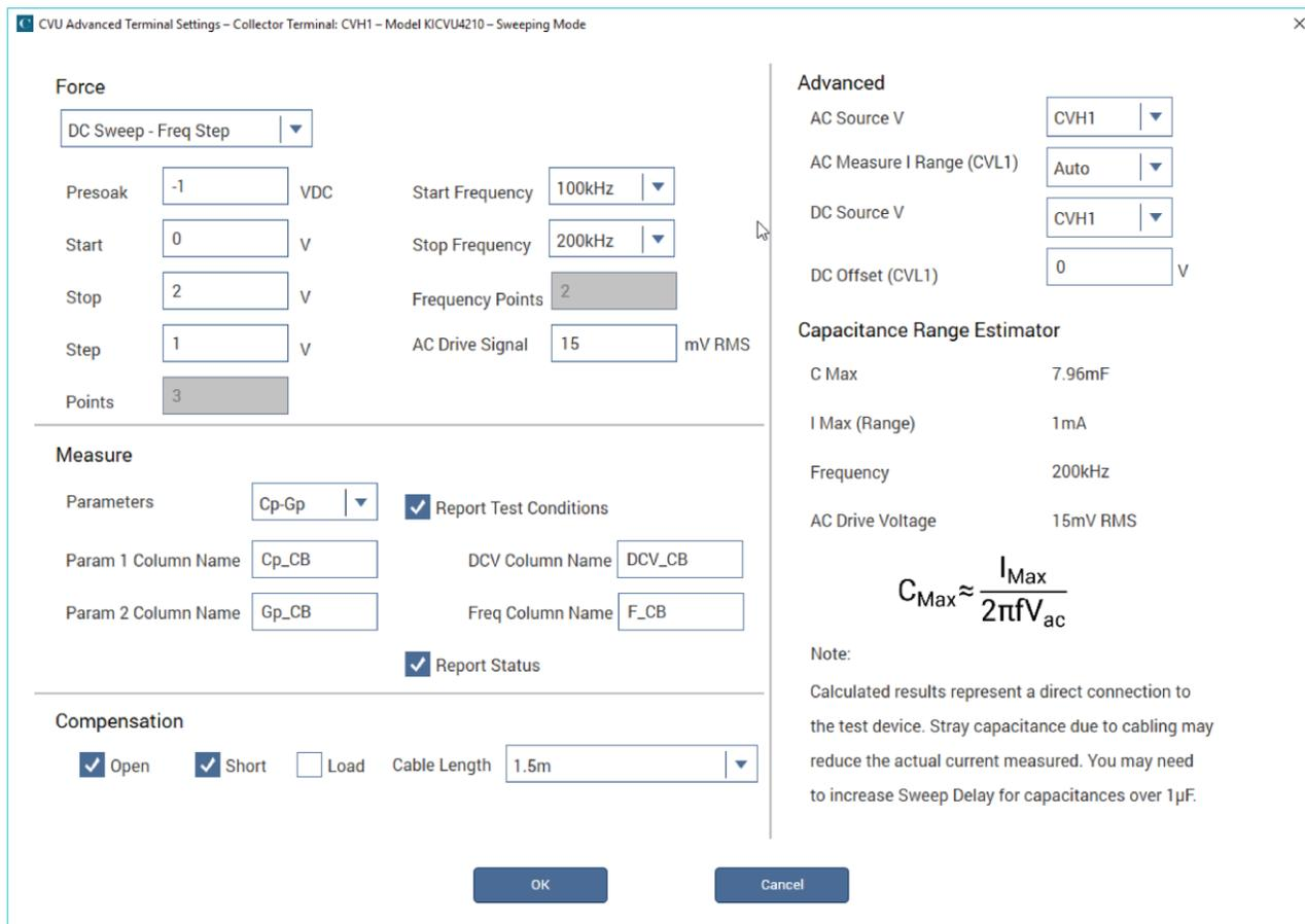
Figure 116: CVU (4215) DC sweep - Freq Step
