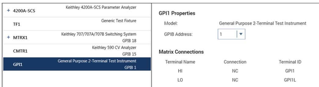
A two-terminal general-purpose instrument is an unsupported external instrument with two terminals (HI and LO), such as a current source. Generally, the instrument HI and LO terminals transmit or receive the instrument stimulus signals.
