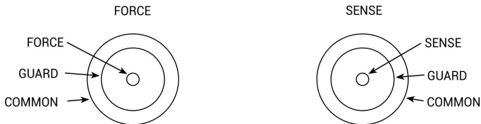
The next figure shows the triaxial cable connections to the device under test (DUT). Note that GUARD is not connected in this example, but it can be routed internally to a test fixture, as described in [Test fixture guarding](#) (on page 3-34).
