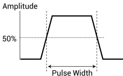
The maximum pulse width that can be set depends on the selected period for the pulse. For example, if the period is set for 500 ns, the maximum pulse width that can be set for the fast speed is 490 ns (500 ns – 10 ns = 490 ns).
