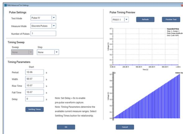
Select **Preview Test** to animate the waveform. The cursor moves from left to right on the bottom graph while displaying the point waveform of each sweep within the cursor on the top graph.
