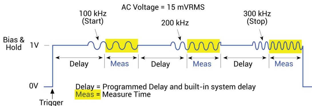
CpGp is measured on each frequency step of the sweep.
