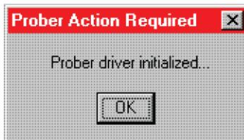
4. Issue a `PrChuck` command to tell the user to ensure that the first test site is ready for testing. The `PrChuck` dialog box opens and the user continues by clicking **OK**. Tests on the site are executed.
