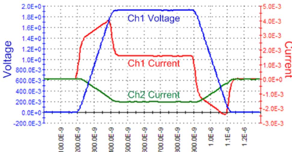
The previous figure shows the current waveforms for both PMU channel 1 (high side) and channel 2 (low side) current measurements. Note that channel 2 does not show the capacitive charging effects. Also, note that the channel 2 current measurement is negative because the current is flowing into channel 2.
