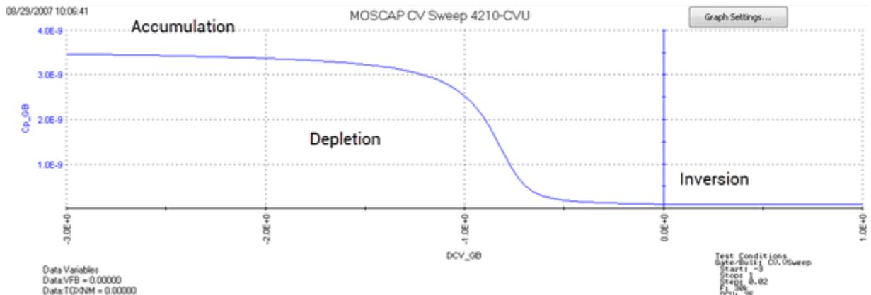
The C-V curve for an n-type MOS capacitor is analogous to a p-type, except that:
