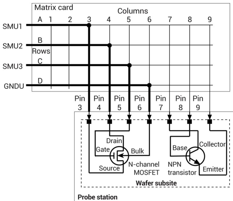
5. The test runs `vds-id-1x`, which generates a family of curves ( $I_D$  vs.  $V_D$ ) for the MOSFET.
