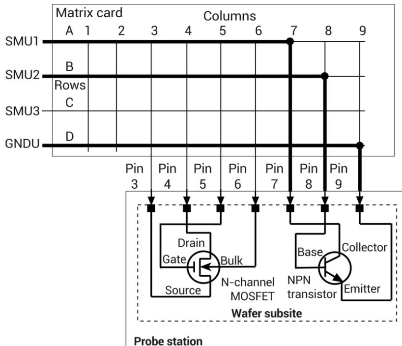
8. The test runs `vce-ic-1x`, which generates a collector family of curves ( $I_C$  vs.  $V_C$ ) for the transistor.
