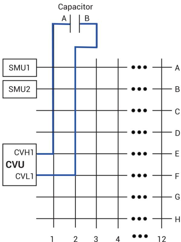
This project is set up for use with a Series 700 with a 7174A matrix card. You must configure the switching system and the matrix card in KCon (see [Add an external instrument](#) (on page 7-4) in the KCon section). Make sure sensing is set to Local (2-wire).
