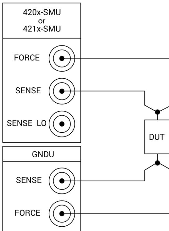
Figure 53: Full-Kelvin preamp - ground unit connections
