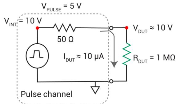
This example shows a 5 V pulse into a 1 MΩ DUT load.
