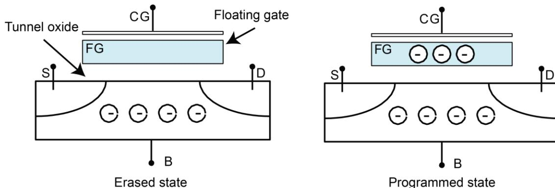
The control gate (CG) reads, programs, and erases the FG transistor. The presence of charge on the gate shifts the voltage threshold ( $V_T$ ) to a higher voltage, as shown below.
