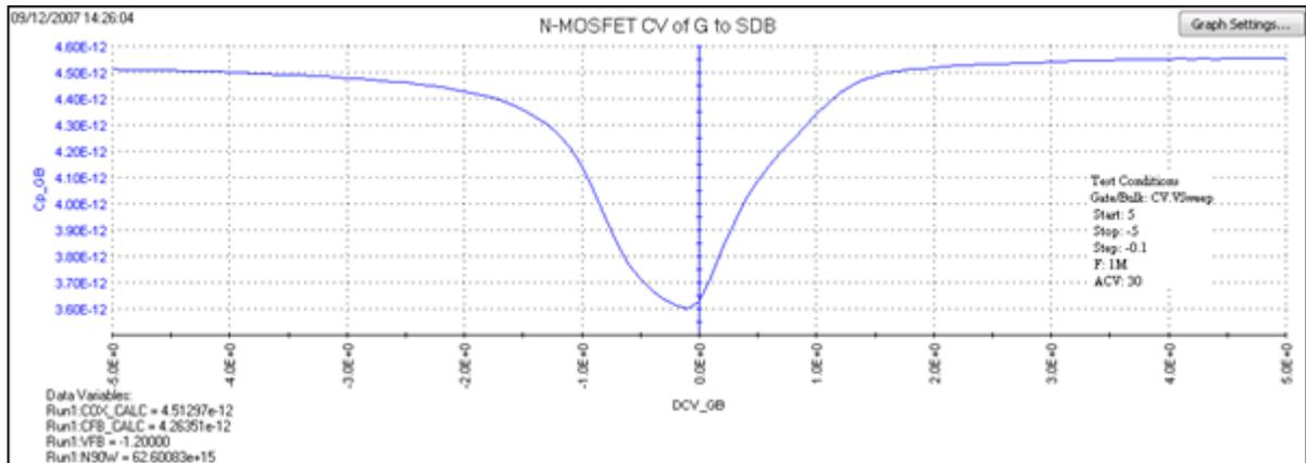
Notice from the high frequency curve that when the device is in the inversion region, the capacitance is high, unlike the MOS capacitor, which has low capacitance in inversion. This is because the MOSFET has a source and drain, which enables inversion charge to flow, unlike the MOS capacitor, which relies on generation and recombination in the bulk region.
