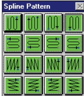
3. Select the spline pattern. The icon of the active spline pattern is transferred to the Edit Die Program Parameters dialog box, as shown in the following figure.
