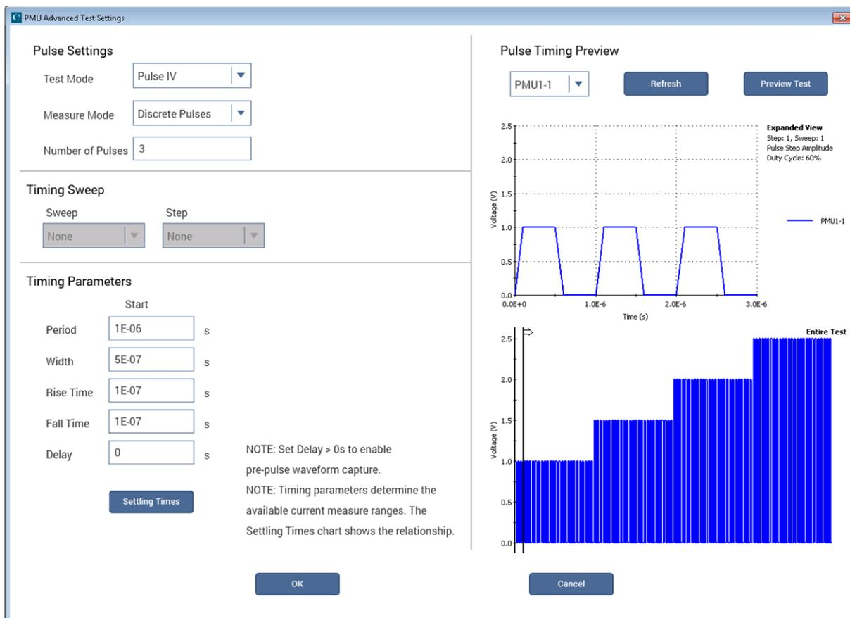
Configuring the preview to all channels displays both the sweeper and stepper for the three-pulse test (see next figure).
