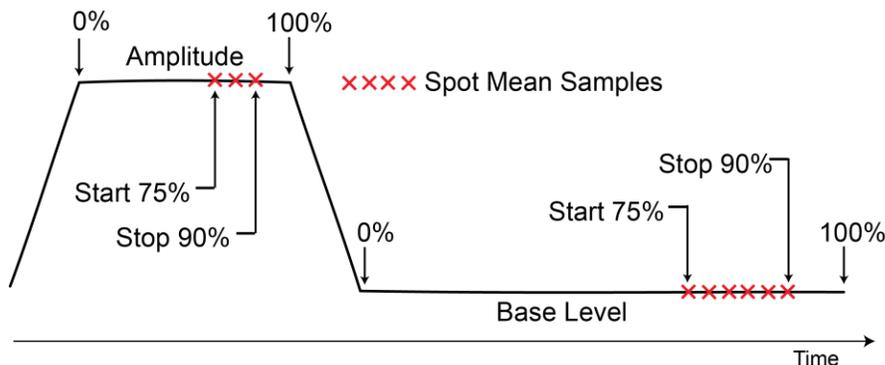
The number of measurement samples that are made is relative to the widths of the magnitude and base level. For example, if the width of the magnitude is 1  $\mu$ s, the measure window is 750 ns to 900 ns. If the width of the base level is 2  $\mu$ s, the measure window is 1500 ns to 1800 ns.
