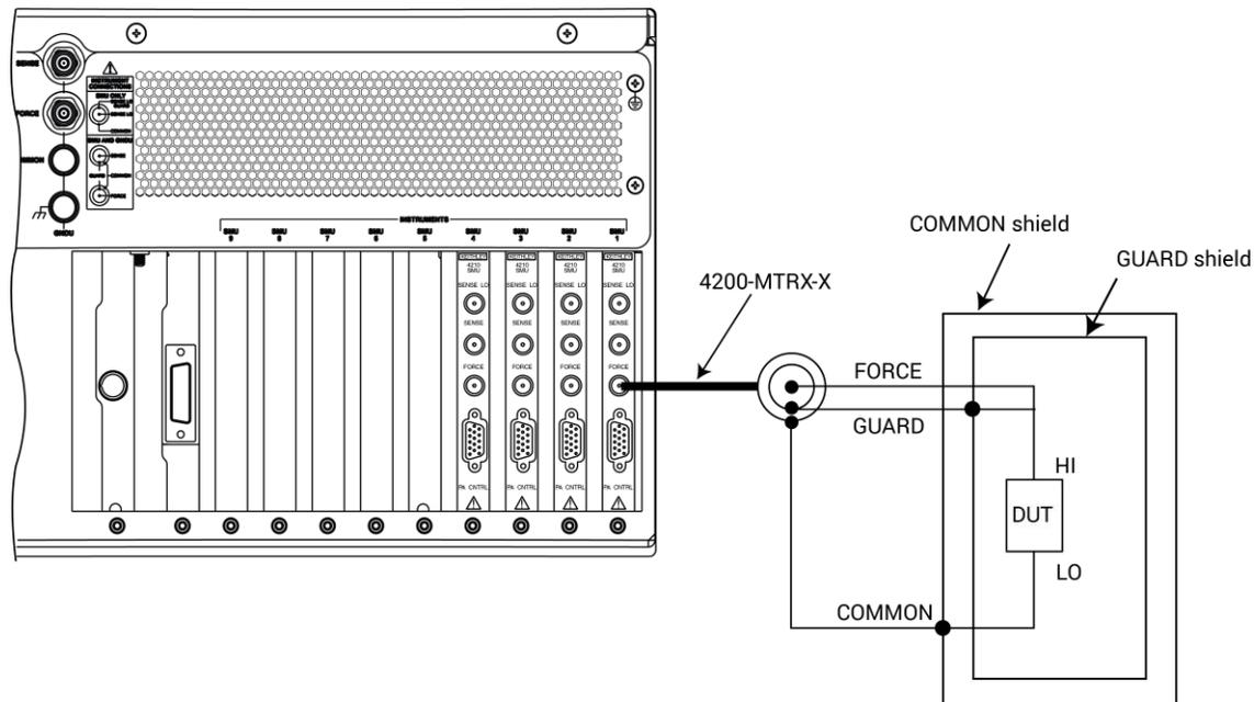
Figure 5: Device guarding basic circuit
