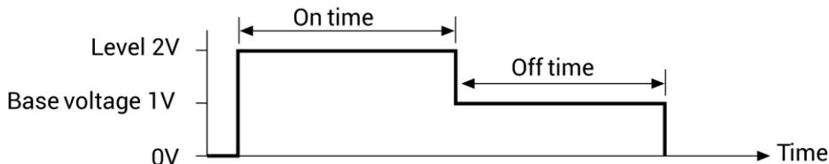
**Pulse Mode: 3-step linear voltage sweep (no measure)**
