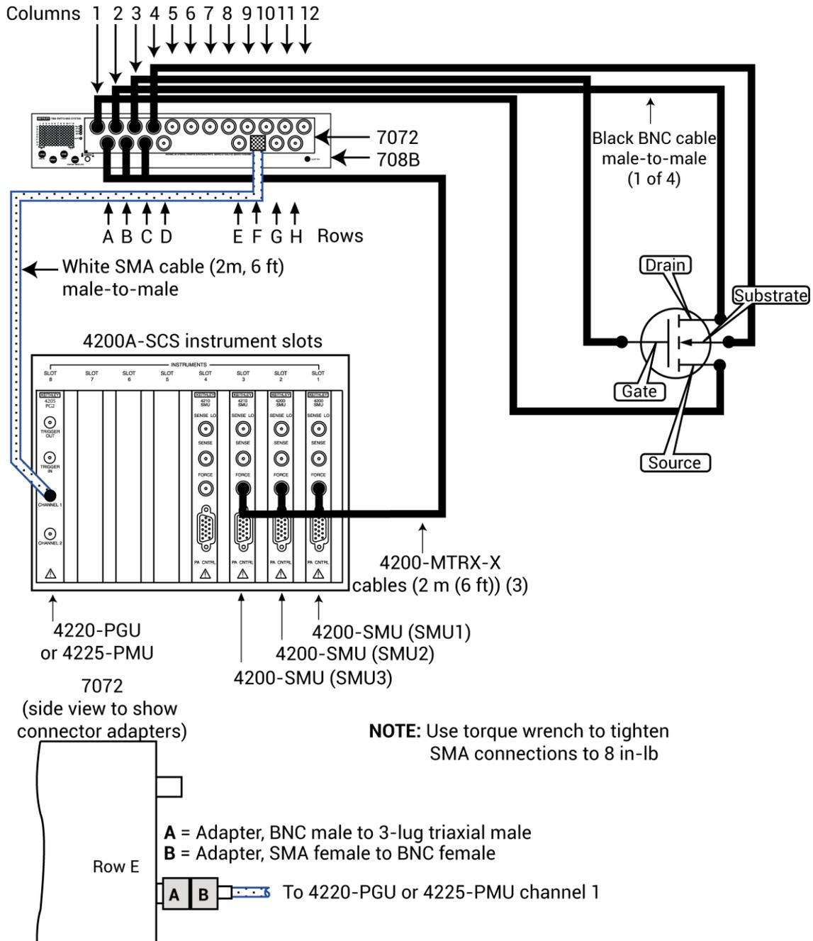
**NOTE:** Use torque wrench to tighten SMA connections to 8 in-lb
