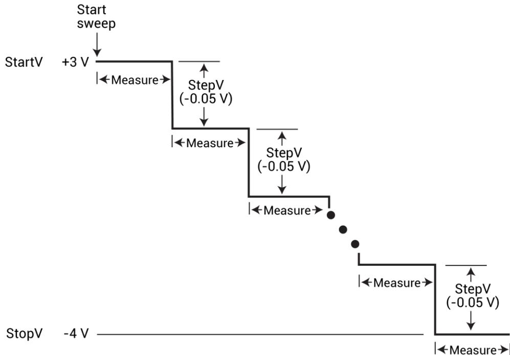
A typical graph that is generated by this test is shown below.
