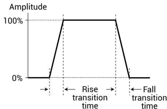
The pulse rise time setting takes effect immediately during continuous pulse output. Otherwise, the rise time setting takes effect when the next trigger is initiated. The `pulse_trig` command is used to trigger continuous or burst output.
