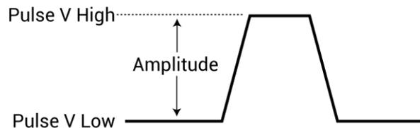
The pulse voltage low setting takes effect immediately during continuous pulse output. Otherwise, the voltage low setting takes effect when the next trigger is initiated. The `pulse_trig` command is used to trigger continuous or burst output.
