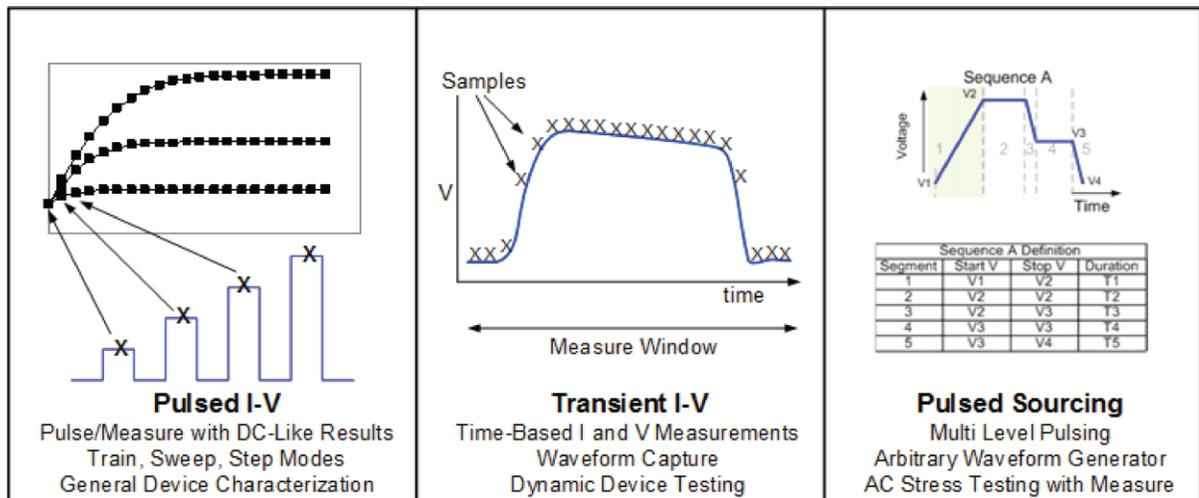
"Pulsed I-V" refers to any test with a pulsed source and a corresponding high speed, timed-based measurement that provides DC-like results. The current, plus voltage measurement, is an average of readings taken in a predefined measurement window on the pulse. This average of readings is called the "spot mean." You can define the parameters of the pulse, including the pulse width, duty cycle, rise and fall times, amplitude, and so on.
