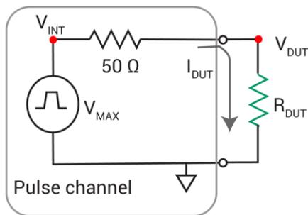
As shown in the figure, the voltage across the DUT,  $V_{DUT}$ , is directly related to the resistance  $R_{DUT}$ . The discussion here is simplified, including resistive impedances only.
