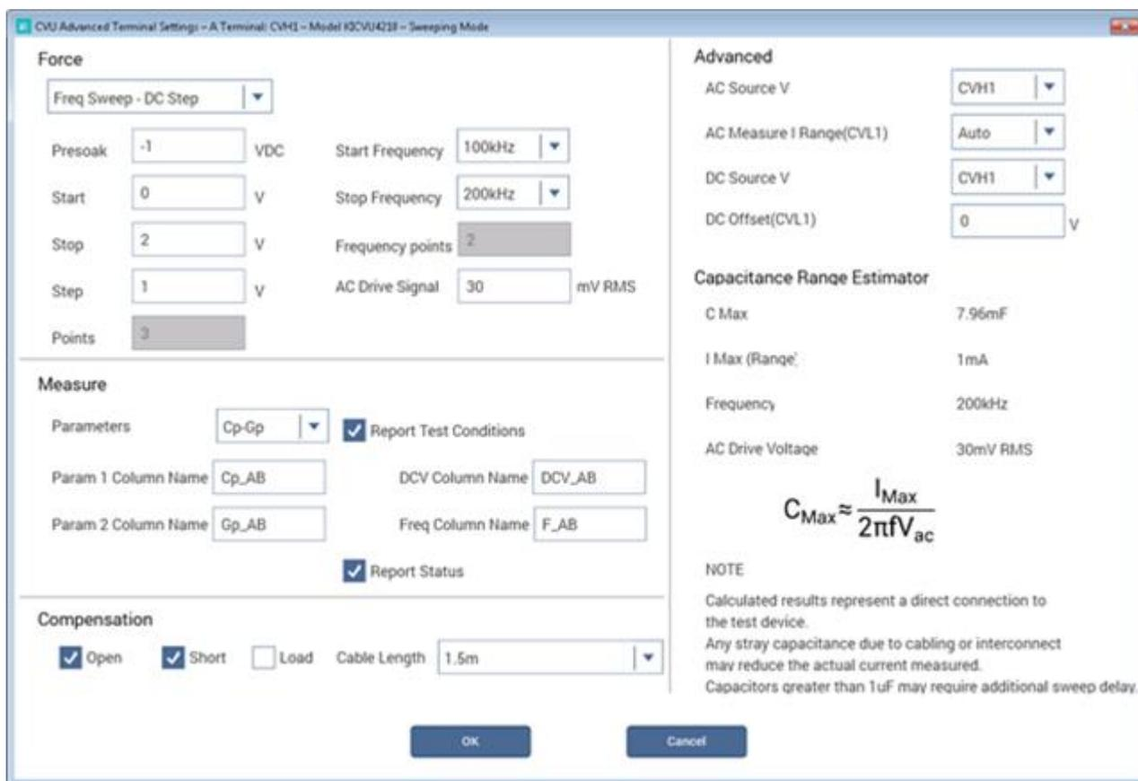
Figure 113: CVU (4215) Freq sweep - DC step
