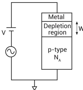
**Figure 143: Reverse-biased p+n junction**
