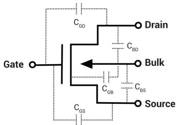
C-V measurements are often made on MOSFETs to extract particular device parameters, such as oxide capacitance ( $C_{ox}$ ), flatband capacitance ( $C_{FB}$ ), and oxide thickness ( $T_{ox}$ ).
