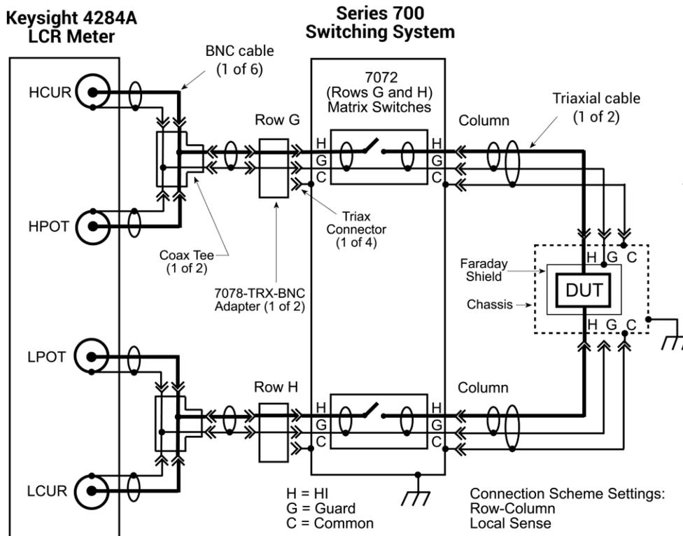
The next figure shows the remote sense signal paths for the Keysight Model 4980A LCR meter through a 2-pole matrix card. Since row pairing is required, the remote sense setting must be used.
