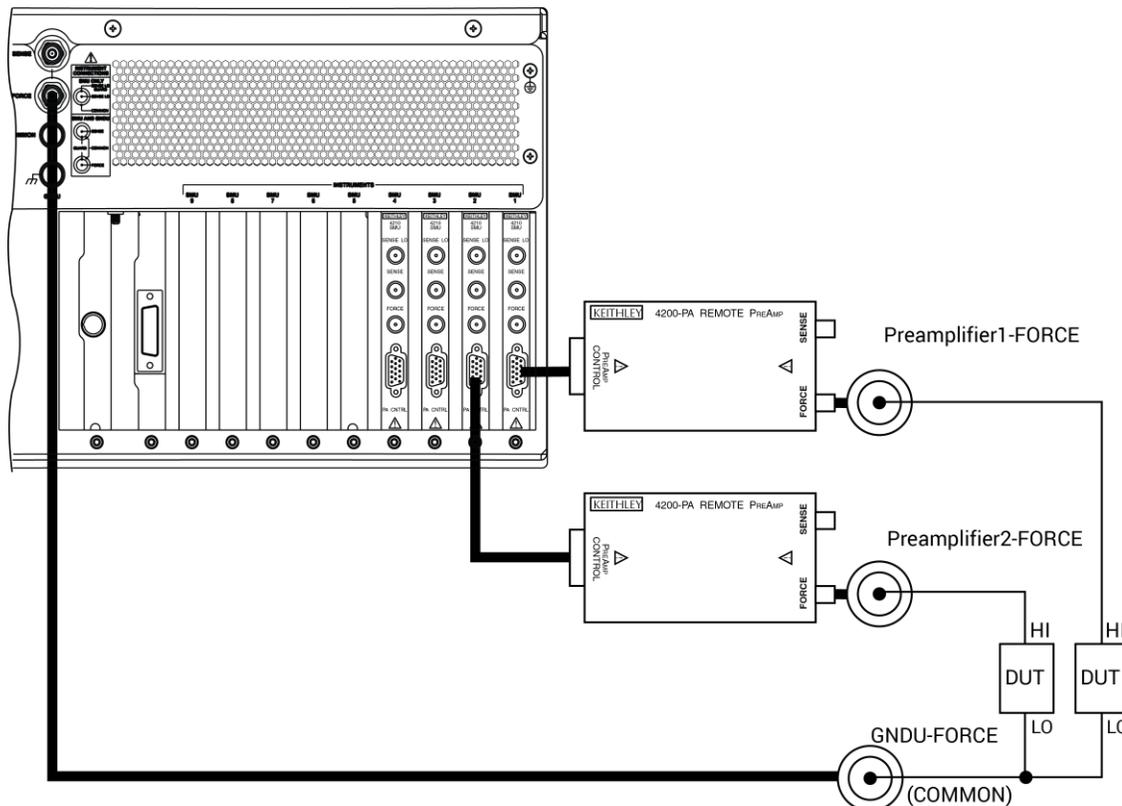
Figure 16: Ground unit and Preampifier local sense connections schematic
