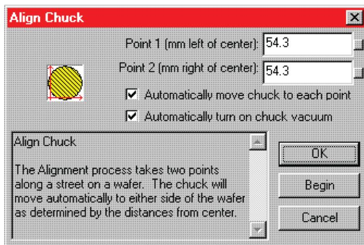
If the alignment is not correct, repeat the alignment. If the alignment is correct, click **Finish**.
