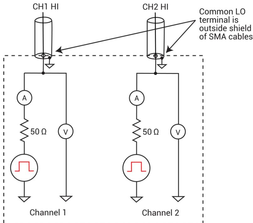
Because pulsing requires high frequency signal propagation, reduce cable inductance by minimizing the loop area of the connection to the device under test (DUT). See the next figure and the following figure for a graphic definition of the loop area for the coaxial cabling.
