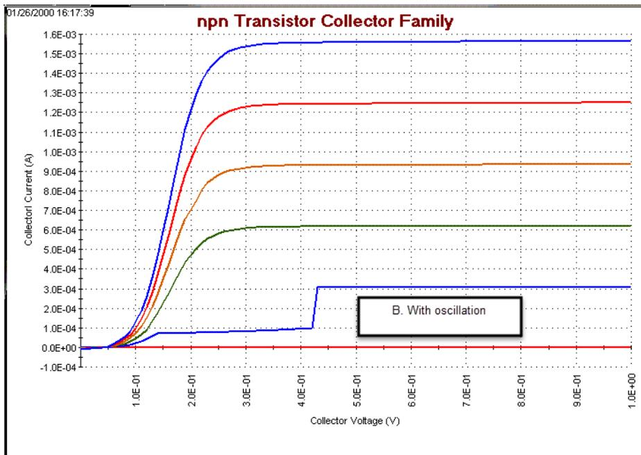
In general, oscillations can be classified in two categories: high-frequency oscillations (100 kHz through 200 MHz), and low frequency-oscillations (below 100 kHz). For solutions to both types of oscillation, refer to [Eliminating oscillations](#) (on page 13-11).
