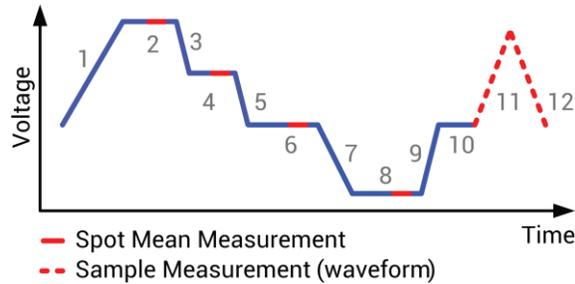
Two types of measurements are supported: spot mean and sample. Spot mean measurements take a mean of all the samples within the measured window and result in a single reading for that segment. The sample measurement reports all of the samples within the measurement window, which can then be plotted versus time to provide a waveform.
