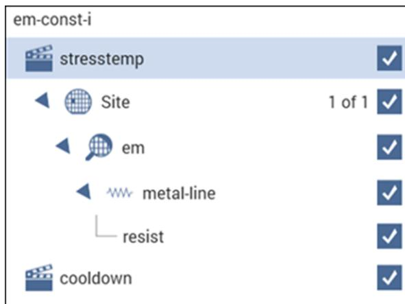
The subsite (`em`) is configured for subsite cycling using current stressing on a single device (`metal-line`).
