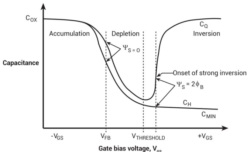
**Figure 708: C-V characteristics of n-type material**
