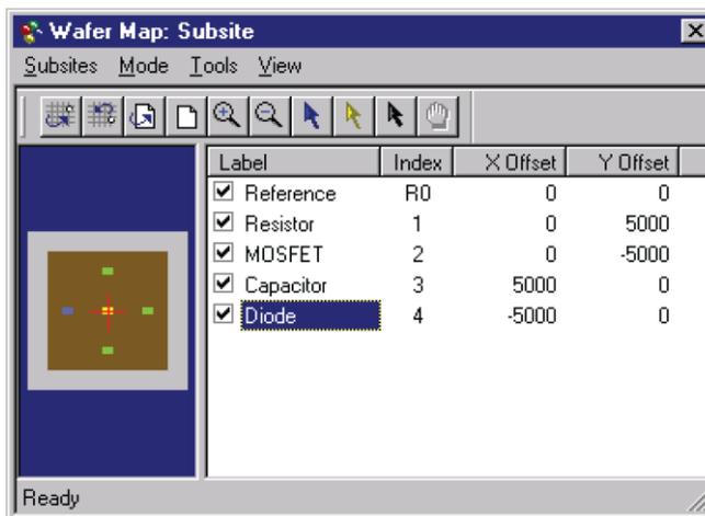
10. To choose a subsite for testing, select the box at the front of each label. To skip testing the subsite, clear the box at the front of each label.
