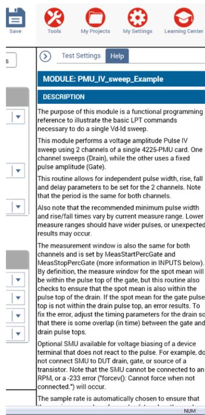
This user module allows for an optional SMU to DC bias a transistor bulk while performing a pulse I-V sweep with a 4225-PMU and optional 4225-RPM. However, due to system restrictions, this SMU must not be connected to the test device through the 4225-RPM (an error results).
