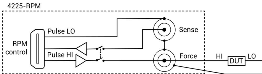
The next figure shows the diagram for remote sensing. Both Sense and Force are connected to DUT HI.
