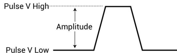
The pulse voltage high setting takes effect immediately during continuous pulse output. Otherwise, the voltage high setting takes effect when the next trigger is initiated. The `pulse_trig` command is used to trigger continuous or burst output.
