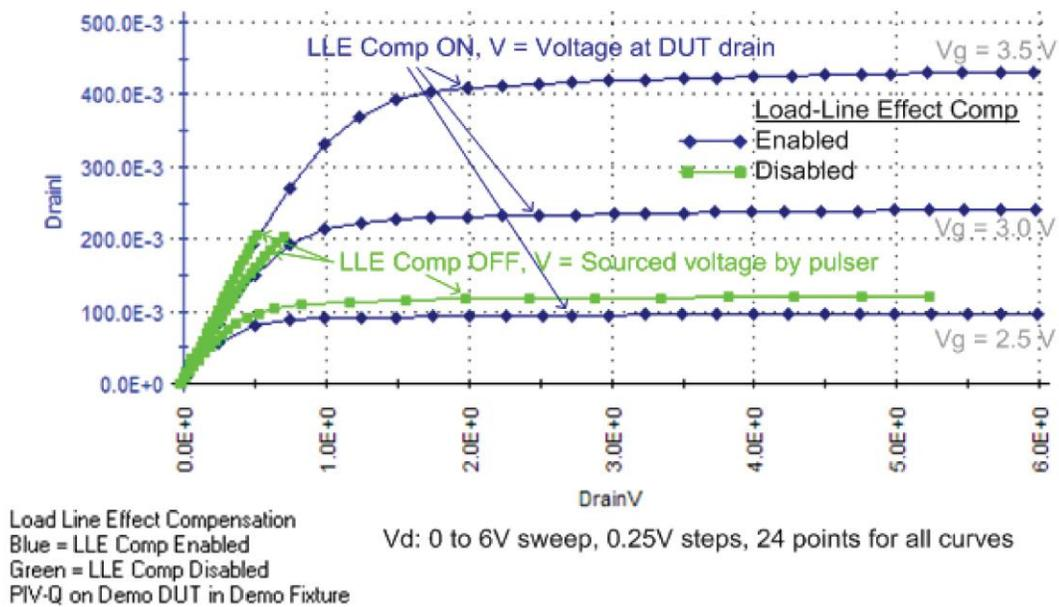
In the previous figure, each blue curve (LLEC on) is the result of a sweep from 0 to 6 V using 250 mV steps. Notice that the 24 pulse-measure points are evenly spaced.
