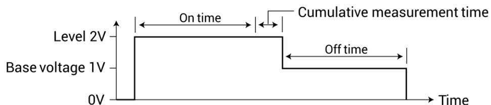
When a measurement is made, it effectively increases the on time by the amount of time required to make the measurement.
