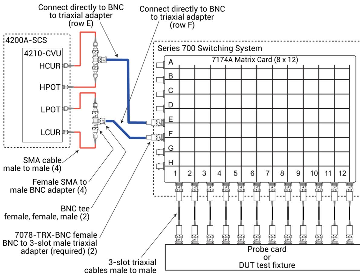
The following figure shows connections for remote (4-wire) sensing.
