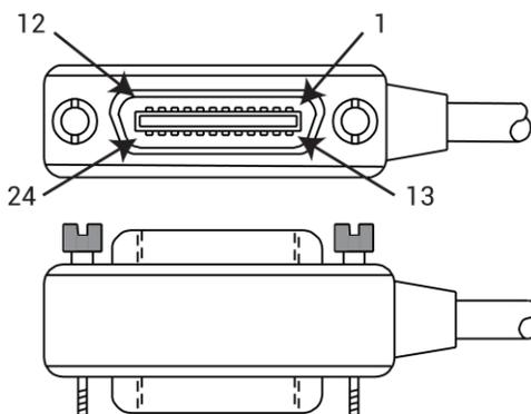
**GPIB control connector terminals**
