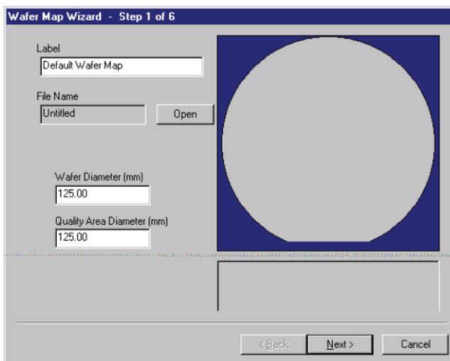
5. Enter the label and wafer diameter in the Wafer Map Wizard window.
