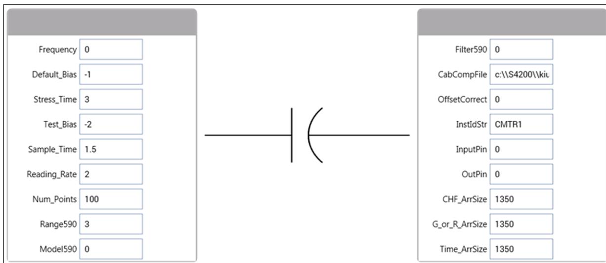
The analog filter, enabled with *Filter590*, can minimize the amount of noise that appears in the readings. It does, however, increase the measurement time.
