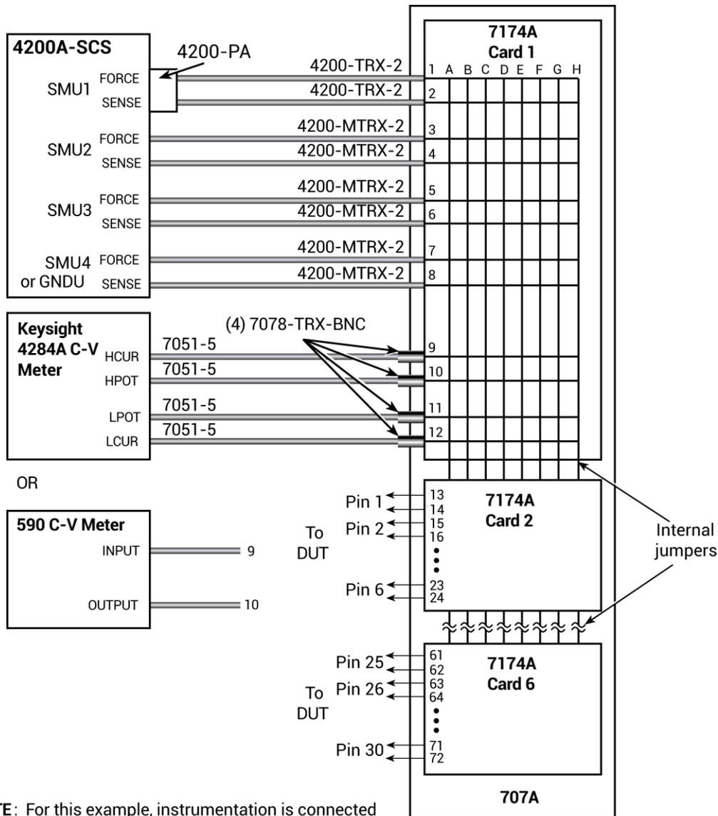
**NOTE:** For this example, instrumentation is connected to matrix columns. Therefore, the switch matrix is rotated 90° for illustration purposes.
