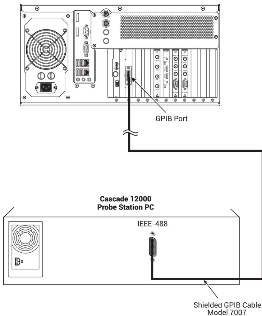
**For probers using the Velox prober control software:**
