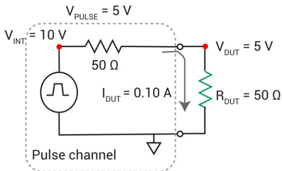
Example 1, showing a 5 V pulse into a 50 Ω DUT load.
