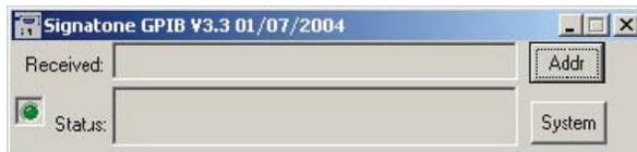
4. Click **Addr** and verify that the GPIB address matches the `GPIB_Address` setting in the 4200A-SCS prober configuration file `prbcnfg_CM500.dat` at `C:\s4200\sys\dat`. Note that the default GPIB address is set to 28.
