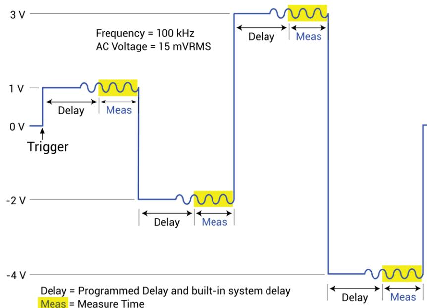
The above figure shows an example of a voltage array sweep using the following voltage values: 1 V, -2 V, 3 V, -4 V. The voltage array is configured as follows:
