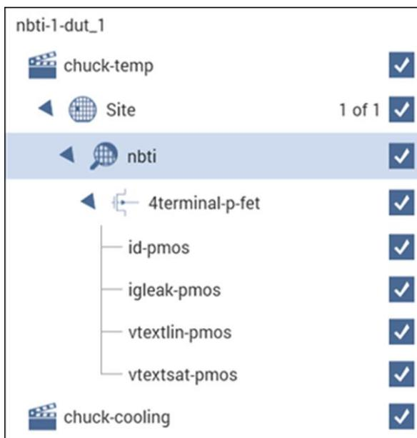
The `nbt_i` subsite is configured for subsite cycling using voltage stressing for a p-channel MOSFET (PMOS) device.
