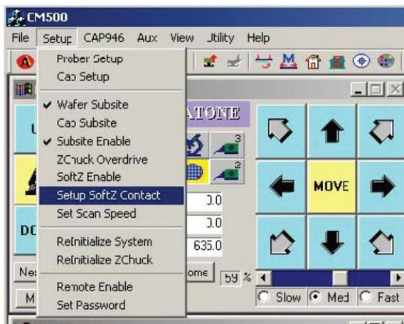
2. Follow the instructions on the window to adjust the height of platen and to determine the contact position of the Z Chuck.
