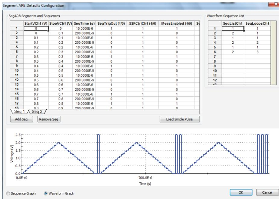
Figure 308: UTM UI Editor Segment Arb Defaults Configuration for channel 2
