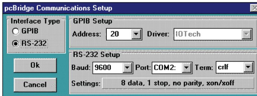
7. Use the pcBridge Communications Setup to configure the communications settings. These settings should be 8 data, 1 stop, no parity, xon/xoff.
