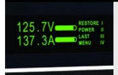
The Model 2001's multiple display capability makes it easy to gather several pieces of information simultaneously from different aspects of a single signal. One of these displays is ideal for power supply monitoring because it shows the DC voltage of the supply's output, the AC noise level, and the frequency of that noise all at once, which simplifies tracking down the source of the noise and correcting it.
