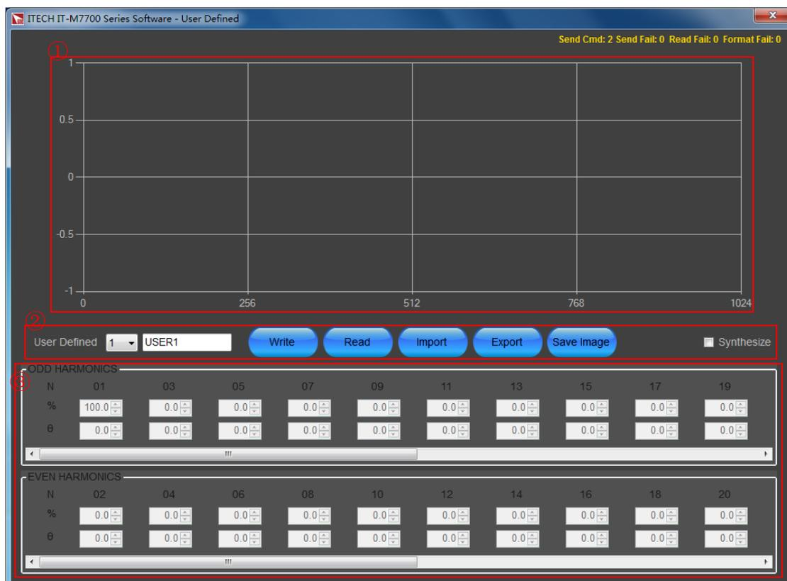
1. Self-defined waveform display zone: display the waveform graph of the real-time self-defined waveform.
