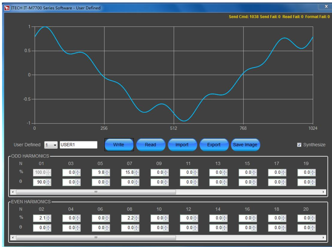
4. Click **Write** button to write the real-time Self-defined waveform into the IT-M7700 instrument. And the IT-M7700 power supply will conduct test based on the Self-defined waveform.
