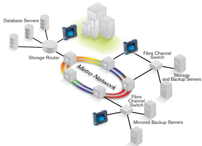
Thanks to end-to-end network testing capabilities, EXFO's FTB-860 enables fast deployment and configuration of Fibre Channel networks. Communication between the transport network, interconnection devices and end nodes can be validated with features such as BER testing, latency measurement, buffer-to-buffer credit estimation and port login capabilities.
