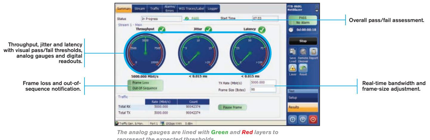
The analog gauges are lined with **Green** and **Red** layers to represent the expected thresholds.
