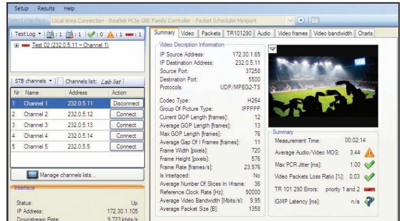
The EXpert IPTV Test Tools allow technicians to emulate an actual set-top box. When operating in that mode, the application can join and leave live IPTV channels. The user can connect and view one or several standard-definition or high-definition videos simultaneously, or request a specific one.
