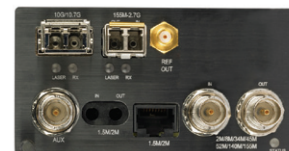
FTB-8130 module with SONET/SDH and OTN test functions.
