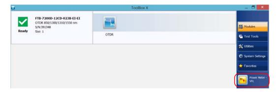
**Note:** The **Power Meter and VFL** button is only visible if your unit is equipped with a power meter and a VFL.
