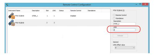
**Note:** If the **LINS** column is empty, it means that the corresponding instrument cannot be controlled using SCPI commands.
