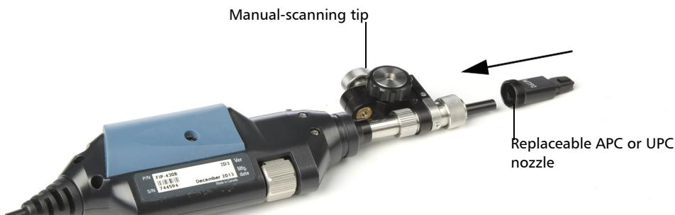
3. Insert the bulkhead adapter on the nozzle.
