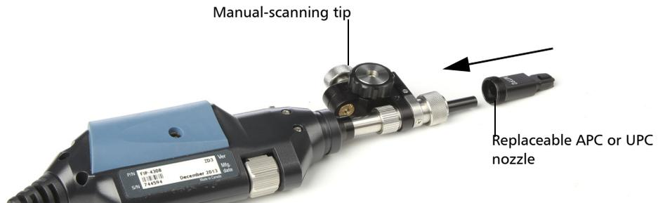
3. Insert the bulkhead adapter on the nozzle.
