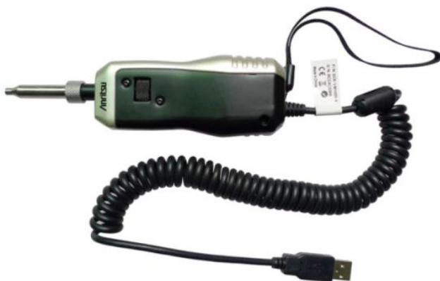
Figure 12-1. Anritsu G0306A Video Inspection Probe
