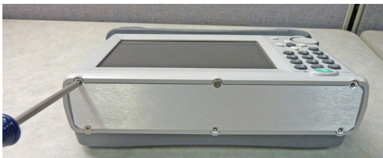
Figure 10-2. Remove the Battery Cover Plate
