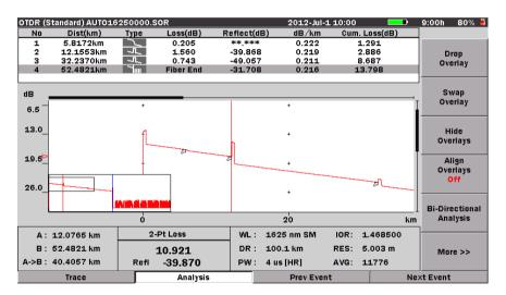
Figure 4-33: Trace Screen with Overlay Traces Hidden
