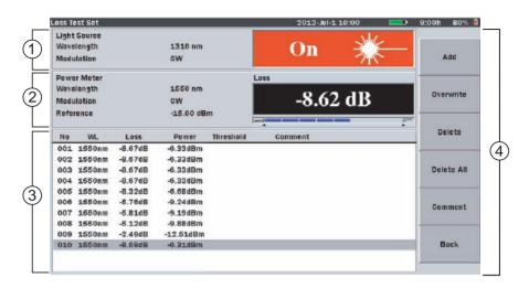
Figure 8-7: Loss Test Set – Loss Table screen
