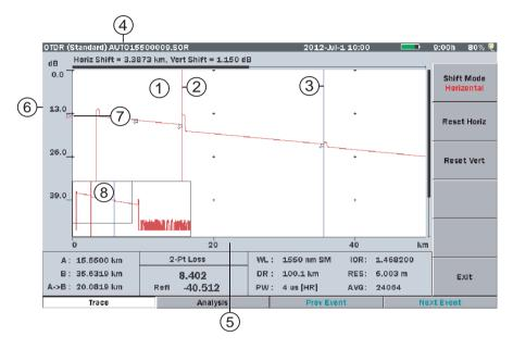
Figure 4-11: Trace Graph – OTDR (Standard) Mode
