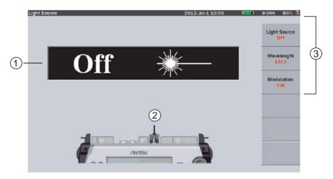
Figure 9-12: Optical Light Source Screen Elements
