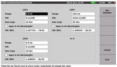
Figure 6-10: OTDR (Construction) Parameters screen
