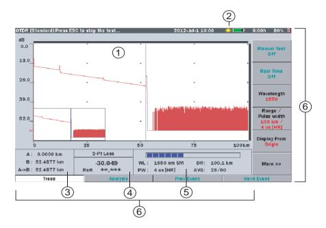
Figure 4-10: Trace Screen with Laser On Indicator
