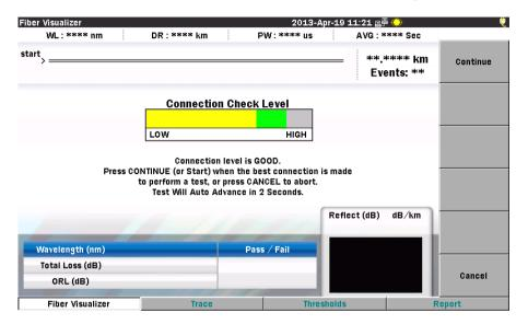
Figure 5-17: Connection Check screen
