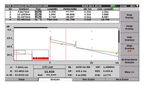
Figure 4-30: Trace Screen with Trace Overlay Softkeys
