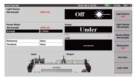
Figure 1-6: Initial Loss Test Set screen
