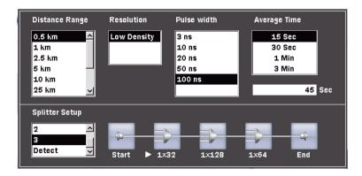
Figure 5-22: Range/Resolution/Pulse Width/Average Time/SplitterSetup Dialog box
