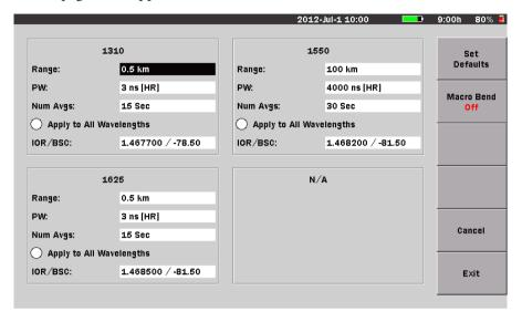
Figure 4-28: OTDR Parameters Screen
