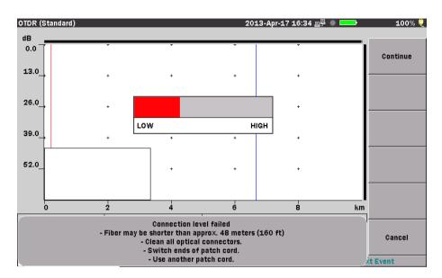
Figure 4-13: Connection Check- Bad Connection
