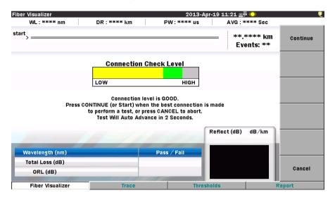
Figure 5-19: Connection Check – Good Connection
