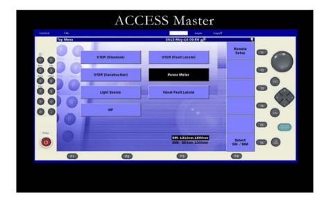
6. A network icon present appears on the upper right of the screen, indicating that unit is now control via Remote GUI.
