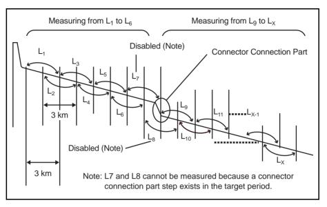
Figure 12-11: Example – When a Fiber (20 km  $\times$  2) is connected
