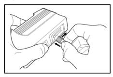
Figure 13-6: Cleaning the Optical Fiber Ferrule End Surface
