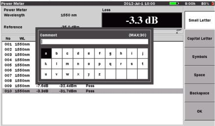
Figure 9-7: Text Entry dialogbox- Loss Test Set mode
