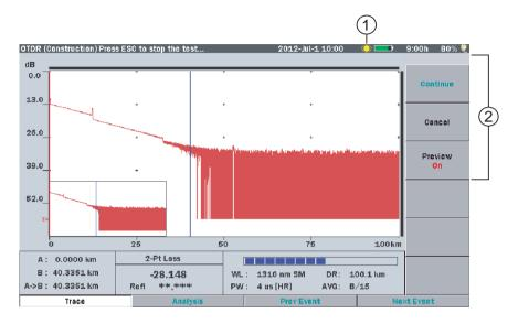
Figure 6-19: Test in Progress screen – OTDR (Construction) mode
