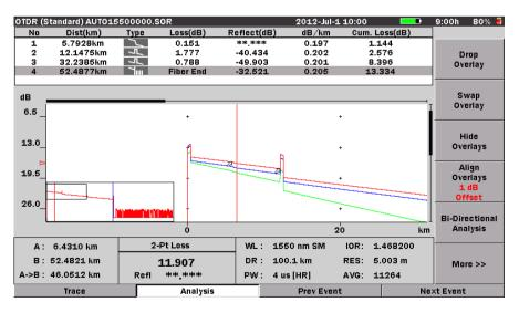
Figure 4-34: Align Overlays 1 dB Offset
