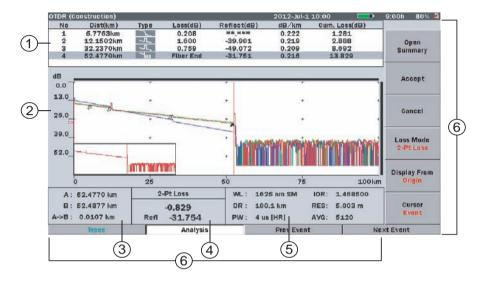
Figure 6-20: Test Results screen with Summary Closed
