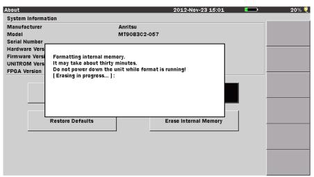
Press Enter to format internal memory or ESC to exit
