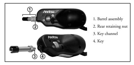
Figure 11-6: Attaching a Probe Tip with Optics
