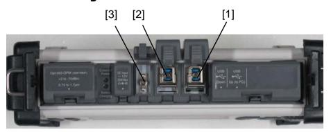
Figure 1: Locations of Laser Beam Apertures
