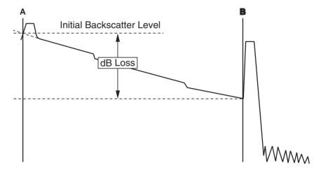
Move Cursor A to the beginning of the fiber and then zoom in on the initial reflection (dead zone). Determine the point where the initial backscatter level would intersect the ascending side of the initial reflection and place cursor A as shown in the figure above. Place Cursor B at the beginning of the reflective end of the fiber.
