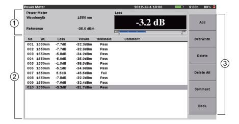
Figure 9-3: Power Meter mode – Loss Table screen
