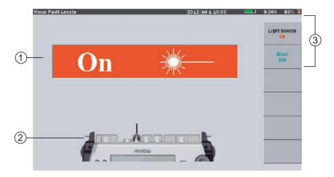
Figure 10-2: Visual Fault Locator On/Off indicator
