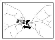
Figure 13-4: Cleaning an Optical Adapter
