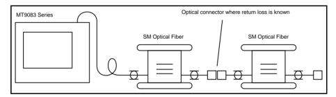
Figure 12-15: Backscatter Coefficient Level Calibration – Connection Diagram
