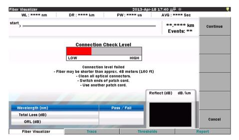
Figure 5-20: Connection Check – Bad Connection
