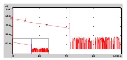
In some cases, such as a very noisy trace or a trace with closely spaced event, you may need to adjust the LSA intervals (fuzzy cursors) to obtain more accurate 2-Point LSA and dB/km LSA loss measurements.
