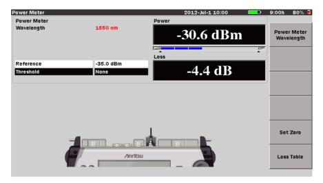
Figure 1-7: Optical Power Meter screen
