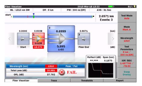
Figure 5-18: Fiber Visualizer Main screen
