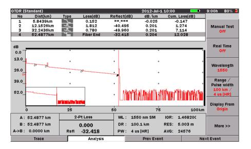
Figure 4-14: OTDR (Standard) Analysis Screen
