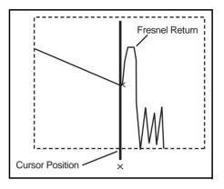
Figure 12-9: Cursor Placement for Distance Measurement Accuracy Test
