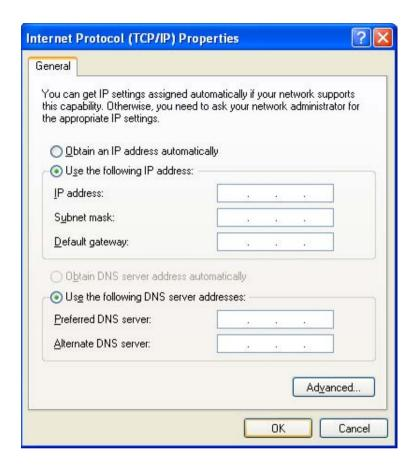
5. For the IP address, assign the network address that is different from the one set for the main unit. In this document, we use the below address. When finished, click **OK**.
