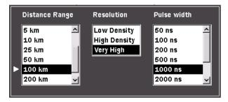
Figure 6-11: Range/Resolution/Pulse Width Dialog box
