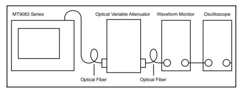
Figure 12-4: Pulse Width Test - Connection Diagram
