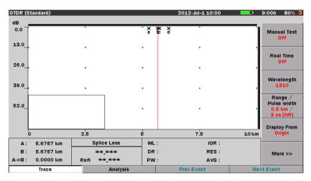
Figure 4-1: OTDR (Standard) Mode – Initial Screen
