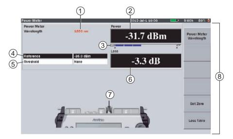
Figure 9-2: Power Meter Screen Elements
