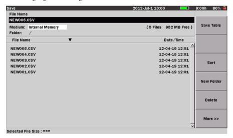
Figure 8-13: Save screen – Loss Test Set mode
