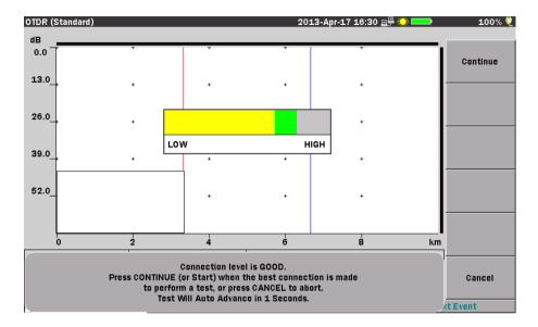
Figure 4-12: Connection Check-Good Connection
