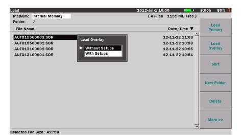
Figure 4-38: Load Overlay Dialog box
