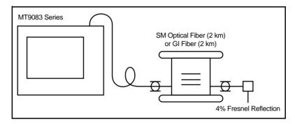
Figure 12-8: Distance Measurement Accuracy Test – Connection Diagram
