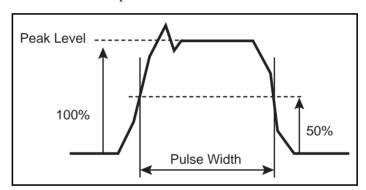
Figure 12-5: Example – Peak Level Half Amplitude measurement
