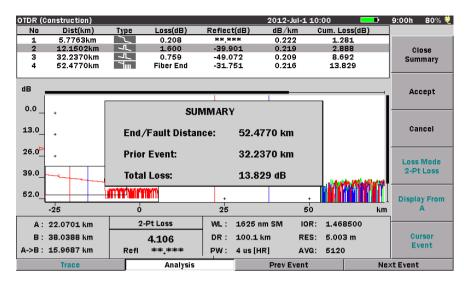
Figure 6-25: OTDR (Construction) Summary screen
