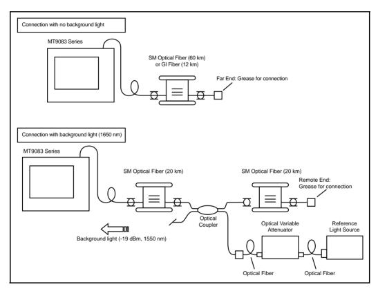
Figure 12-6: Dynamic Range Test – Connection Diagram
