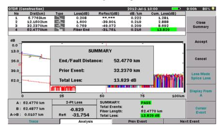
Figure 1-5: OTDR (Construction) Summary screen
