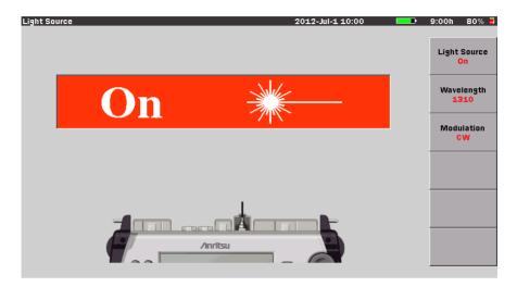
Figure 1-8: Optical Light Source Screen
