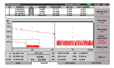
Figure 1-3: OTDR (Standard) Screen with Event Table
