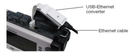
Figure 14-2: Ethernet Cable Connection
