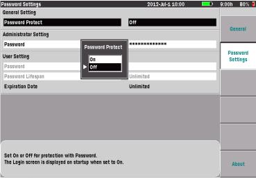
Press the Up/Down keys to move cursor, press Enter or ESC to exit.
