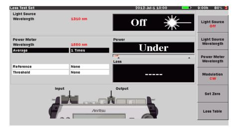
Figure 8-1: Initial Loss Test Set screen
