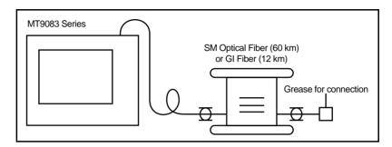
Figure 12-10: Loss Measurement Accuracy (Linearity) Test – Connection Diagram
