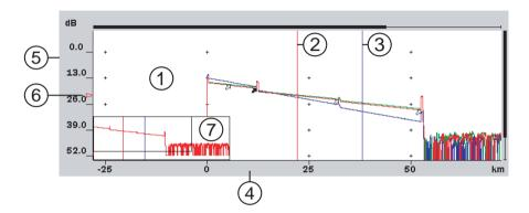
Figure 6-23: Trace Graph – OTDR (Construction) Mode
