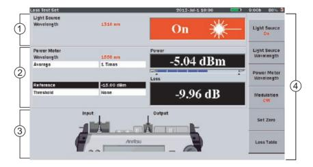
Figure 8-3: Loss Test Set Screen Elements
