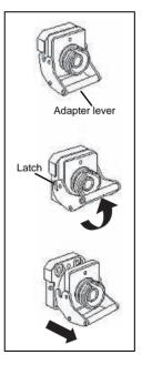
Figure 13-1: Removing the Optical Adapter
