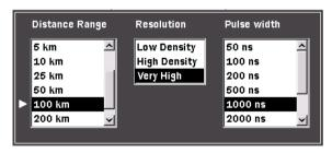
Figure 4-22: Range/Resolution/Pulse Width Dialog box
