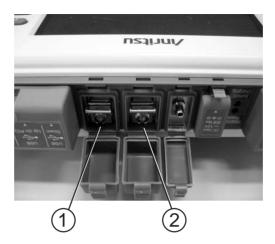
Figure 2-6: Measurement Ports
