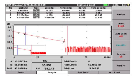
An ORL value with a "<" before the reading and an "S" following the reading indicates that saturation was encountered for the selected area of the trace. This implies that the actual ORL value is, at most, the displayed value, but is probably less.
