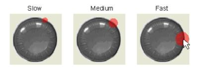
Figure 14-6: Rotary Knob Speed Display
