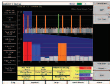
CDMA Code Domain Power measurement display
