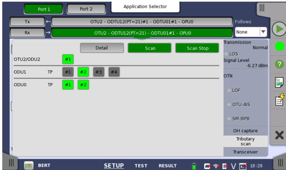
A *Tributary scan* detects errors and alarms over multiple Tributary Ports depending on the current mapping settings at the receiver port. The screen displayed by the **Tributary scan** button can be used to acquire the tributary status information.
