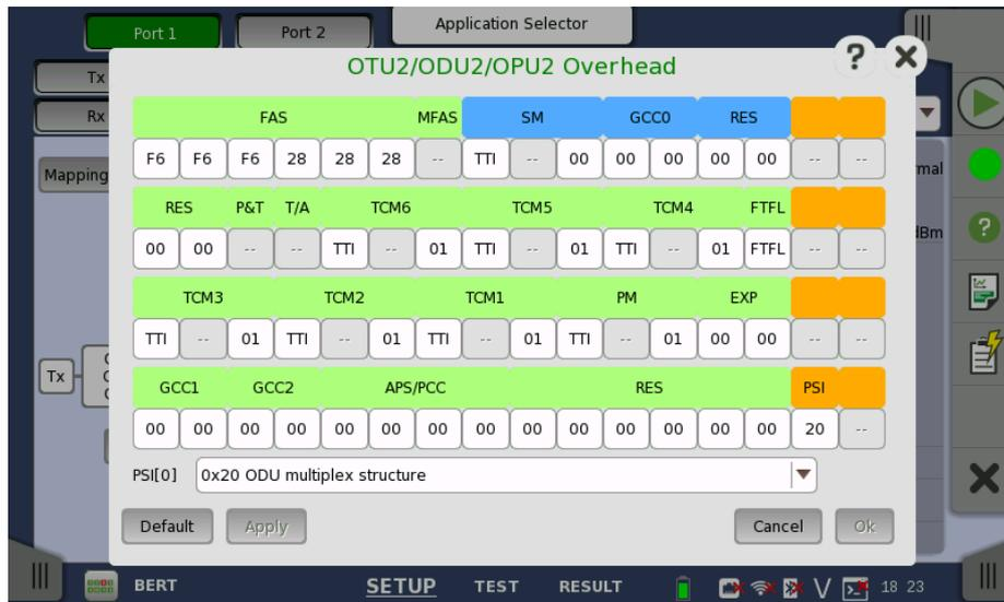
This dialog box presents detailed information about the overhead and allows you to configure it. Blue fields are OTU overhead. Green fields except FAS and MFAS are ODU overhead. Orange fields are OPU overhead.
