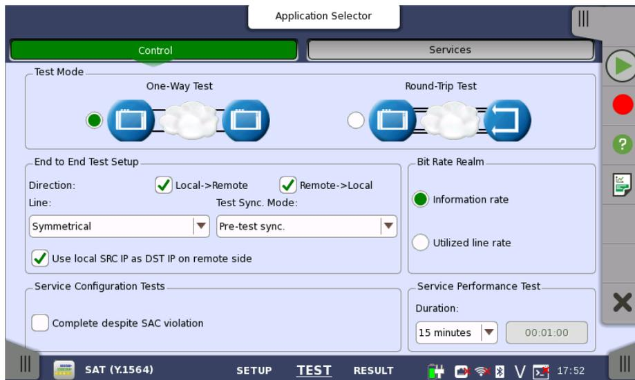
This screen allows you to configure the test mode and other general parameters related to a [Service Activation Test](#).
