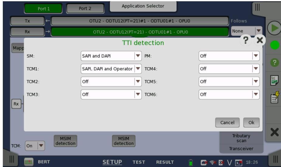
This dialog box allows you to select the detection method for SM, PM, and TCM1-6.
