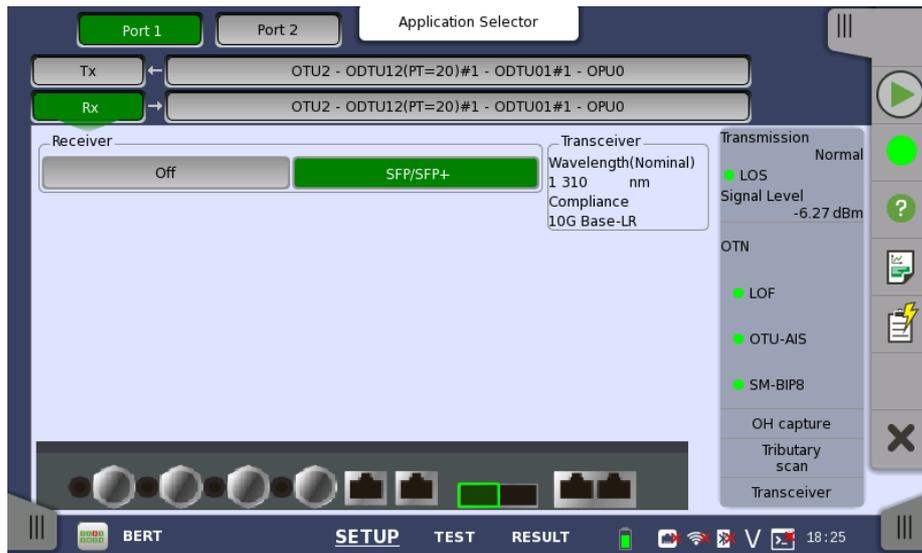
This screen allows you to make the physical setup of the receiver in OTN mode. It can also be used to inspect the current status of the selected port in Port mode lamps.
