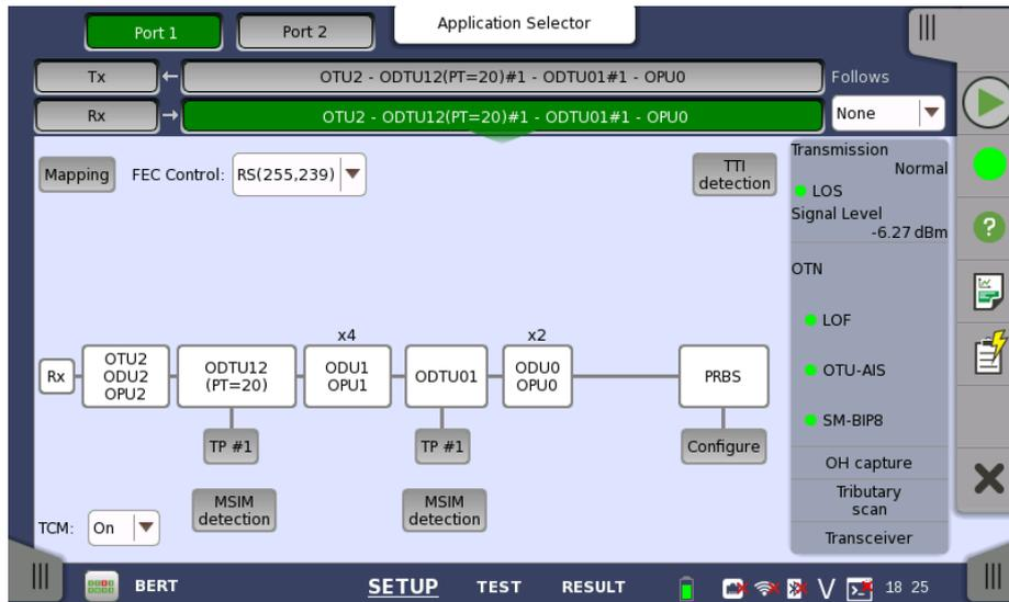
This screen allows you to configure OTUk frame of the currently selected receiver. It can also be used to inspect the current status of the selected port in a separate screen.
