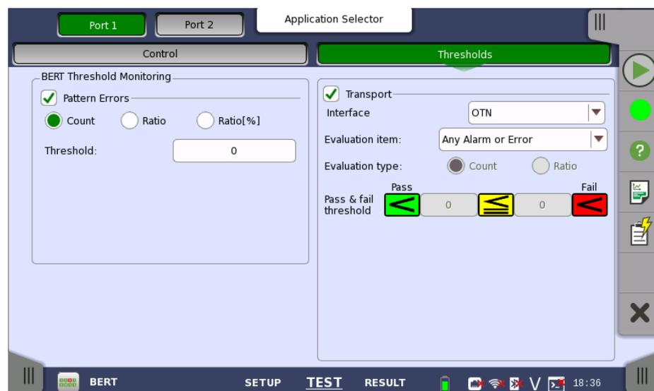
This screen contains the parameters for setting up the various threshold values (i.e. limits) for errors and Pass/Fail status that are used during the monitoring.
