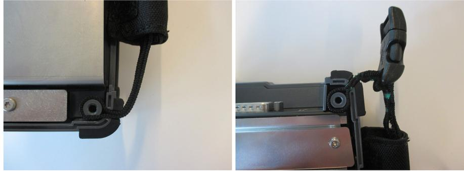
7. Remove the buckle cap from the handle and the carrying strap.
