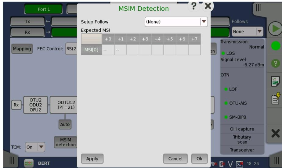
The dialog box is used to set the detection method of MSIM (Multiplex Structure Identifier Mismatch).
