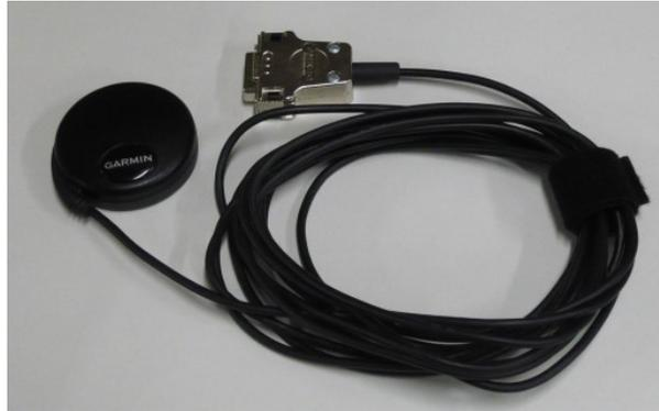
Connect The 15 pin D-sub connector to the 15 pin AUX connector on the connector panel.
