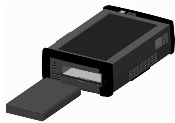
6. When installing the battery, note the direction of the battery terminals. With the instrument placed on its back - and the battery compartment in front of you - the terminals should be in the upper left corner.
