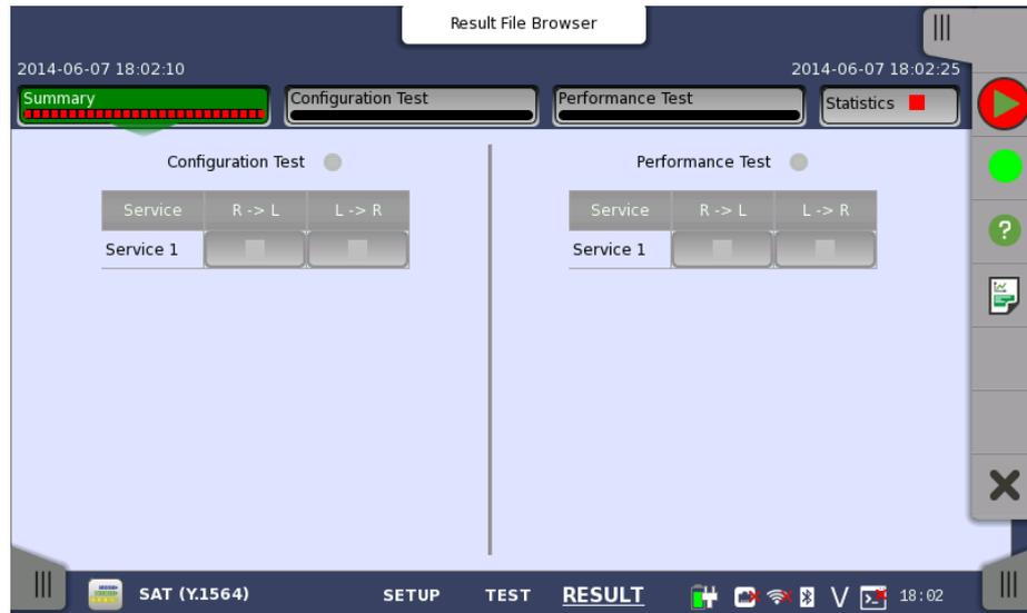
This screen presents a summary of the results of the Service Activation Test. Selecting the result button for a specific service in either the **Configuration Test** or **Performance Test** result panel will display the relevant screen with detailed results information.
