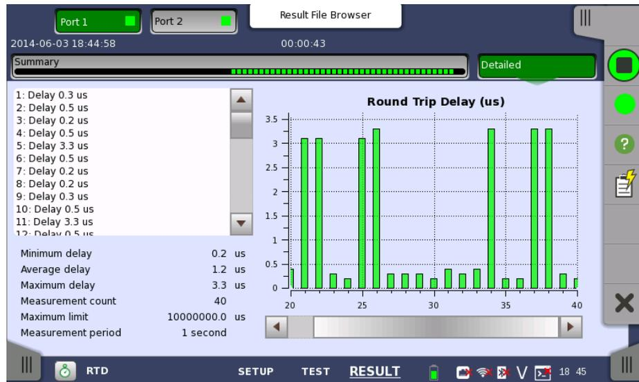
Buttons for selecting the relevant port are displayed at the top of the screen, with a color indication of the pass/fail status of the test.
