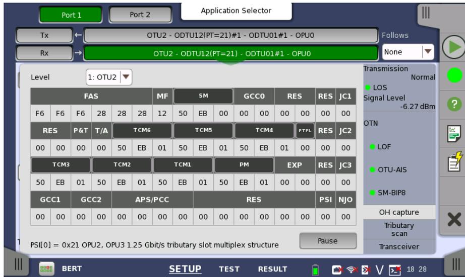
This screen shows OTU/ODU/OPU OH capture data for one frame at time. Use the **Level** drop-down menu to select which multiplexing level to display. For a description of the frame structure, see the [Overhead Dialog box](#) section under the ports setup of OTN.
