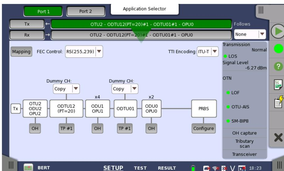
This screen allows you to configure OTUk frame of the currently selected transmitter. It can also be used to inspect the current status of the selected port in a separated screen.
