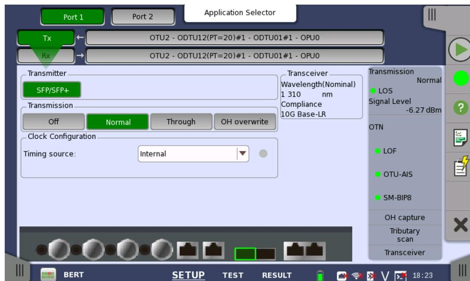
This screen allows you to enable the optical interface of the OTN transmitter. It can also be used to inspect the current status of the selected port in Port Mode lamps.
