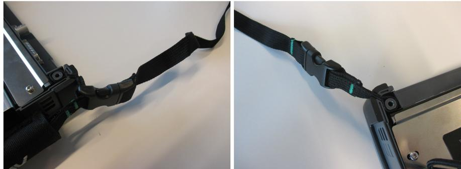
9. Attach MT1000A and MU100010A , insert the battery pack and mount the battery lid with the reverse sequence at the beginning.
