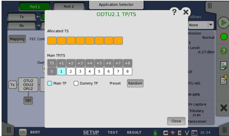
This dialog box allows you to define OTUk frame mapping.
