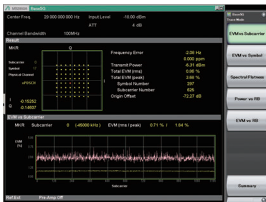
Basic Screen (EVM vs. Subcarrier)
