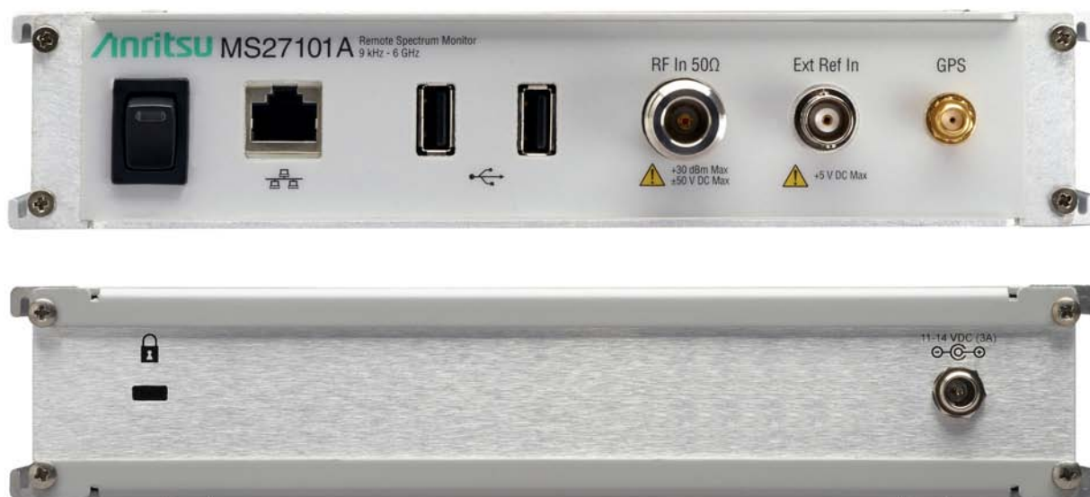
MS27101A Spectrum Monitor
