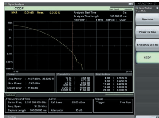
CCDF (Test Model 1, 64 DPCH, 4 Carrier) Waveform Pattern [Test_Model_1_64DPCH x 4]
