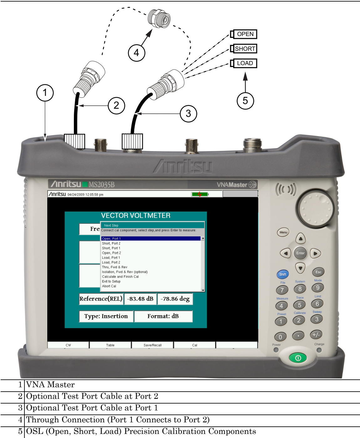
Figure 4-13. 2-Port Calibration (LMR Master and MS20xxB)
