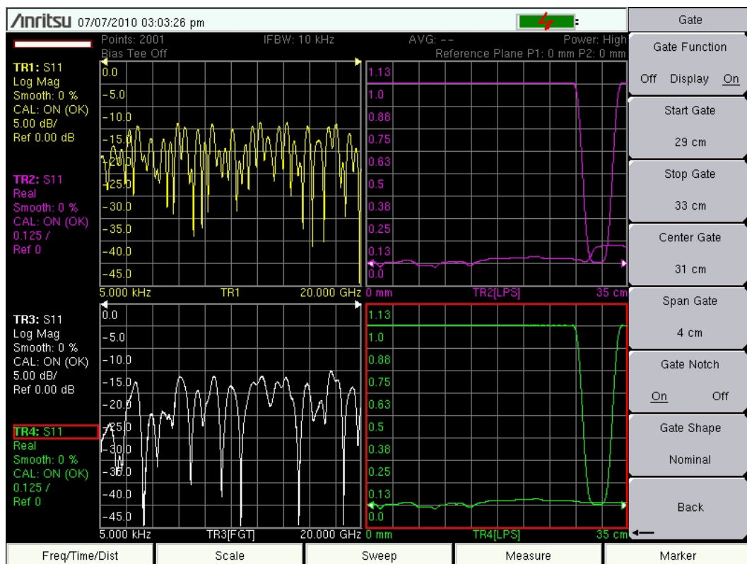
Figure 8-8. DUT at Far End of Cable Measurement – Notch with Frequency Gated by Time
