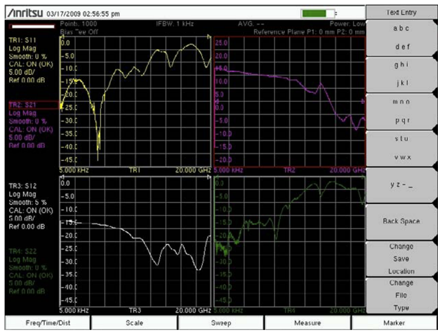
Figure 4-8. Gain, Input Match, Output Match, Isolation of an Amplifier
