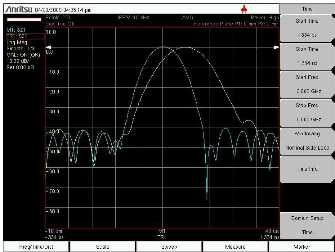
Figure 8-10. S_{21} Measurement of 15 cm Long Waveguide Showing Dispersion Compensation
