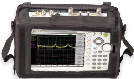
This shows how the case has easy access to test port and other interconnects. A separate flap on the top protects the Ethernet, USB, and power supply connections.
