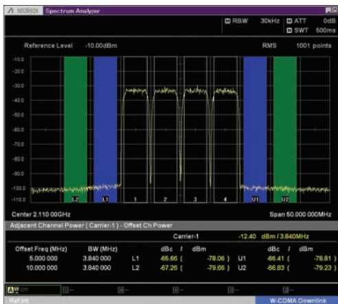
W-CDMA ACLR, 4 Carrier (TestModel1, 64DPCH, 4 Carrier)
