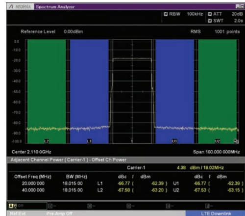
LTE FDD ACLR, 1 Carrier (E-TM1.1, Bandwidth 20 MHz)
