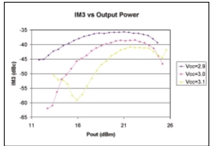
This custom IM3 plot showing third order intermodulation distortion in dBc versus output power for various bias conditions, also involves the Scorpion Navigator orchestrating the IM3 measurement with an external GPIB power supply.
