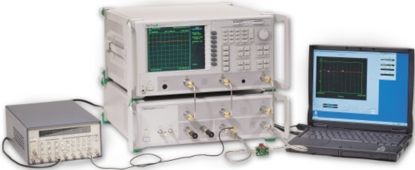
As shown here, the ME7840A also supports pulse measurement conditions (e.g., GSM) when using an external dual pulse generator (as shown here). Using this setup, you can more thoroughly characterize the performance of your power amplifier in terms of match, gain, linearity, efficiency and spectral purity.
