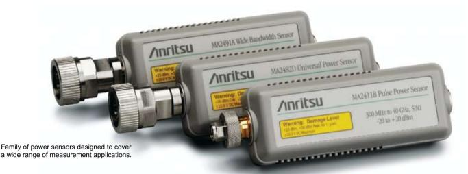
The sensors employ diodes and offer greater speed, sensitivity and dynamic range than thermal sensors. The sensors are based on half or full wave diode rectifiers constructed from zero bias Schottky diodes. The rectifier output is low-pass filtered, forming an envelope detector. This post-detection bandwidth is sometimes referred to as the Video bandwidth and is a measure of how quickly the power sensor can respond to a changing input signal such as a radar pulse or a multi-carrier OFDM signal.
