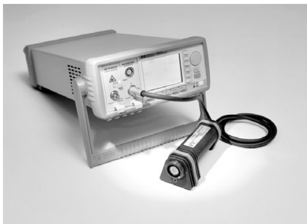
Compact tunable laser source with dual power meter in one box
