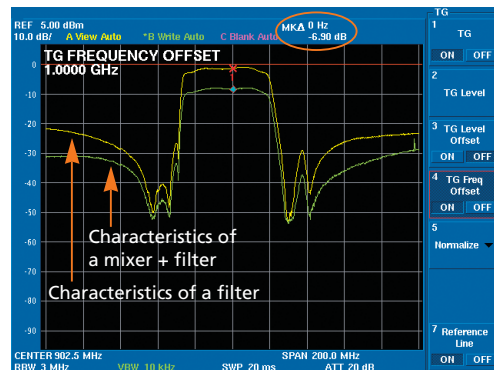
Measurement of mixer frequency conversion loss characteristics
