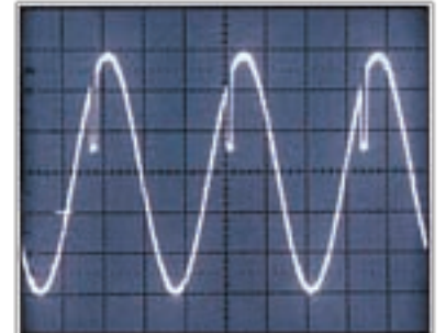
Sine wave with a dropout from 45°-60°.
