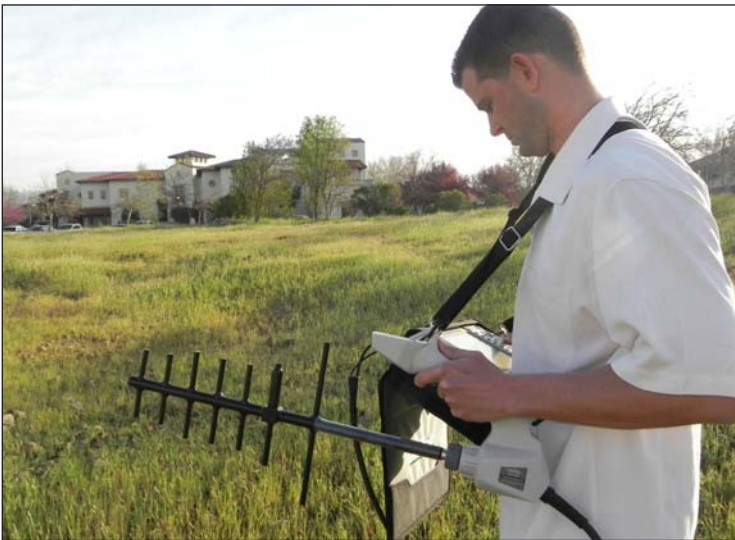
Figure 21: Yagi-antennas are often optimal for signal hunting on foot.
