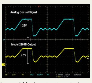
of voltages. They have variable slew rates to create rise and fall conditions. Some models have analog inputs to enable an AC waveform to be superimposed on the DC line for simulation of a noisy line. Many of these features minimize the test instrumentation needed to thoroughly test a DUT.
