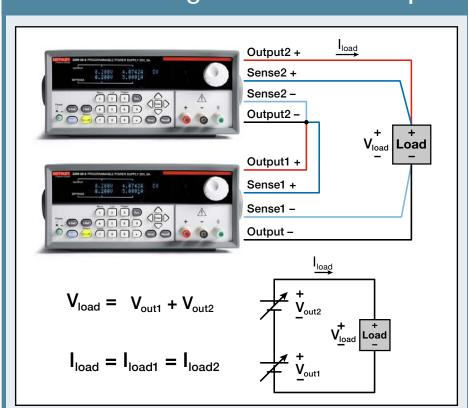
Use several supplies or combine the outputs in a multiple output supply to increase output voltage or current. For multiple output supplies, ensure that all the outputs are isolated; that enables the channels to be combined in either series or parallel. Keithley's multiple output power supplies provide features to simplify controlling and displaying the voltage and current when outputs are connected in series or parallel.
