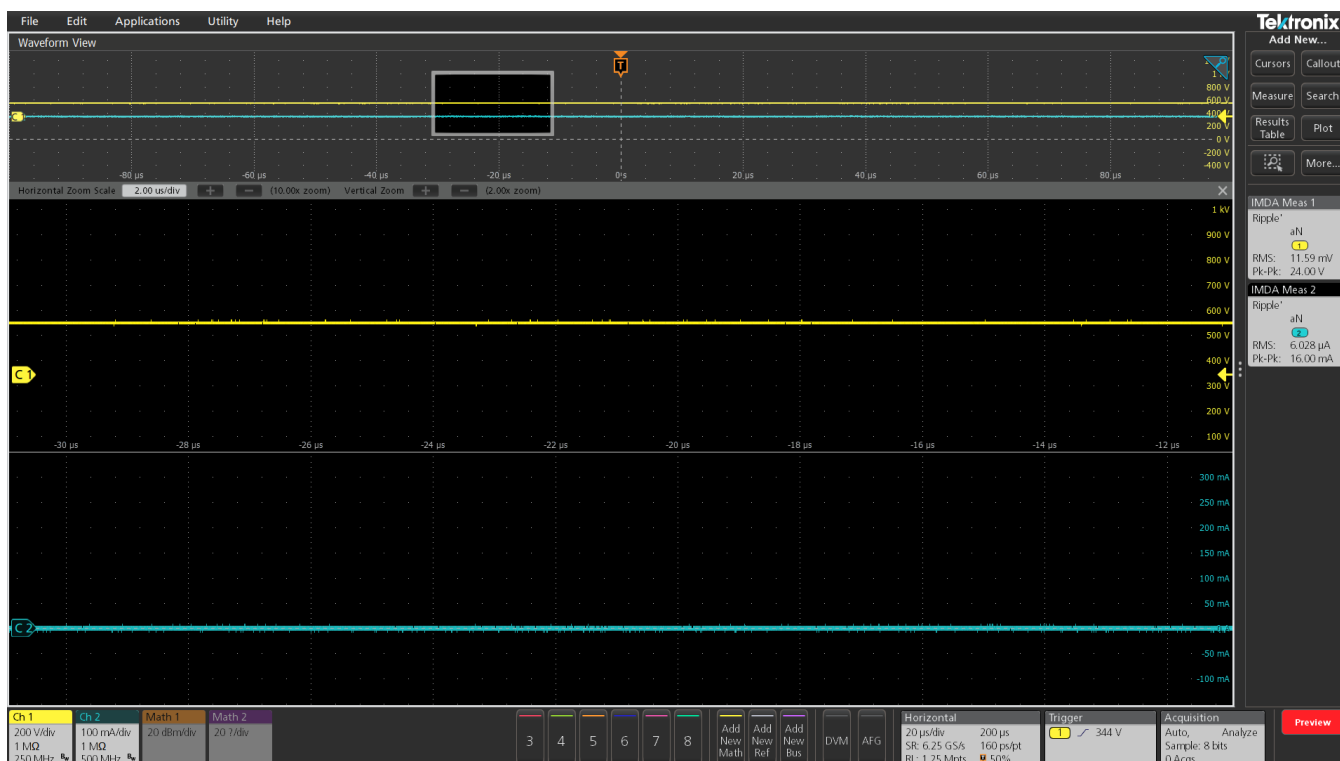
Figure 11: Line Ripple measurement being carried out on the DC-input signals when testing an Inverter
