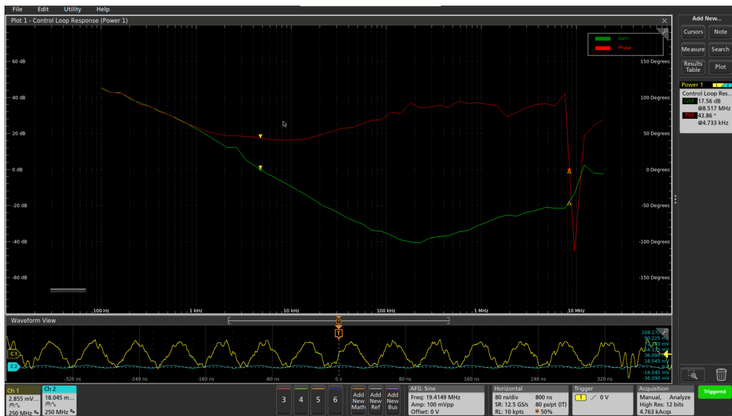
Control Loop Response (Bode plots) plots gain and phase versus frequency and calculates the gain margin and phase margin.
