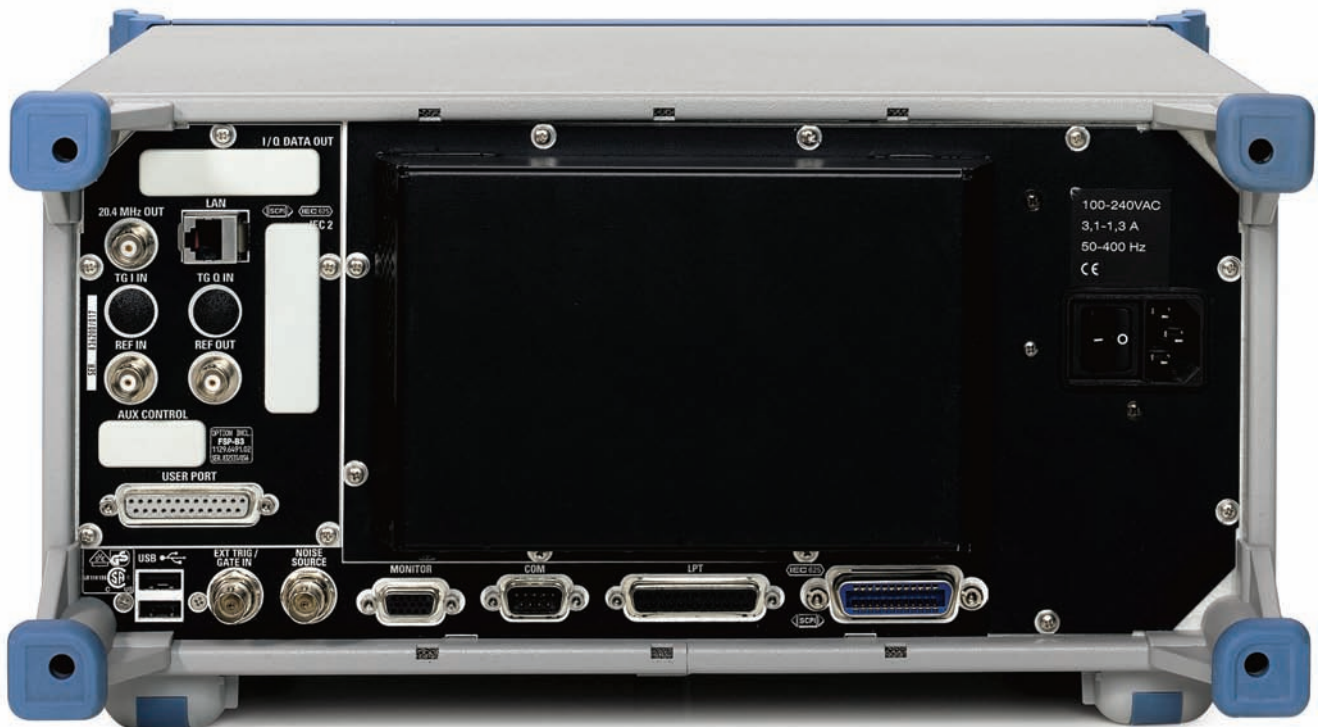
Rear view with interfaces for tracking generator with I/Q, LAN and user port
