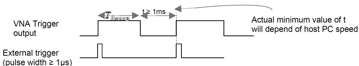
**Note:** The time out value parameter determines when the command is aborted in cases when no external trigger is received. This value is in addition to the built-in default time out which is dependent on parameters such as the bandwidth setting.
