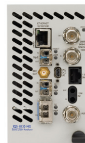
■ IQS-8130NG with next-generation SONET/SDH/OTN hardware including optical and electrical Ethernet add/drop interfaces
