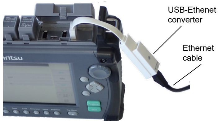
Figure 11.2.1-1 Ethernet Cable Connection
