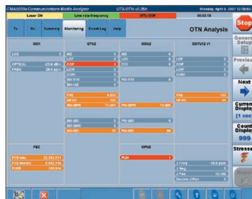
OTN Error and Alarm Display Showing Each Network Layer
